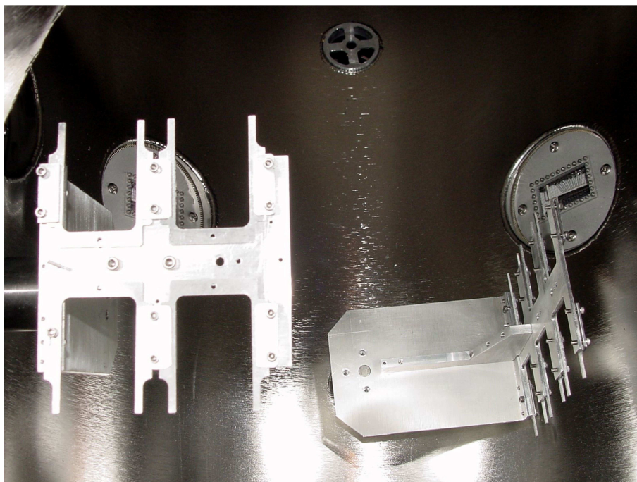
Figure 2.2: The horizontal and vertical target folders viewed from the top of the scattering chamber. The beam goes from the bottom to the top of the picture. (Note this picture is the upgraded one for Run06).
