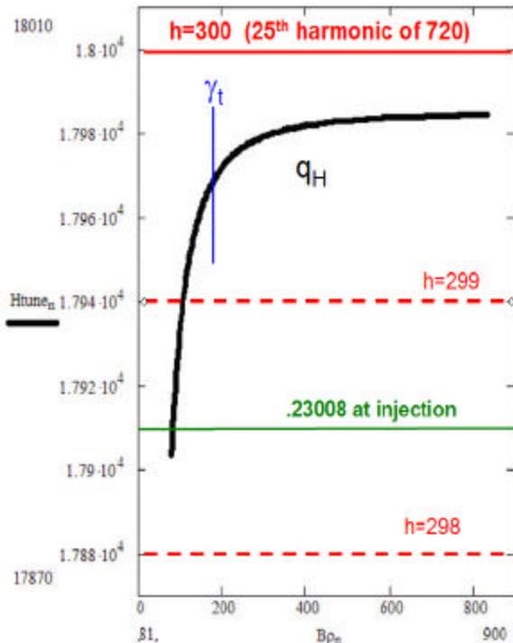
Figure 4: Tune swing up the Au ramp
