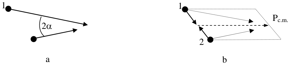
Fig. 3.1. Two particles collision scheme (non-relativistic case) a) – LRF; b) C.M. reference frame
