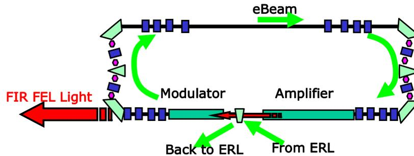
Figure 24: Schematic layout of optics free FEL
