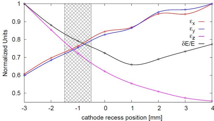
Figure 7: Longitudinal and transverse emittances at the end of a 20 MeV Linac for different positions of the cathode in SRF gun (results of PARMELA simulations). The energy of the  $e^-$  at the exit of the gun was fixed. Note that all emittances are normalized and the solid lines are spline fits to the simulation points.
