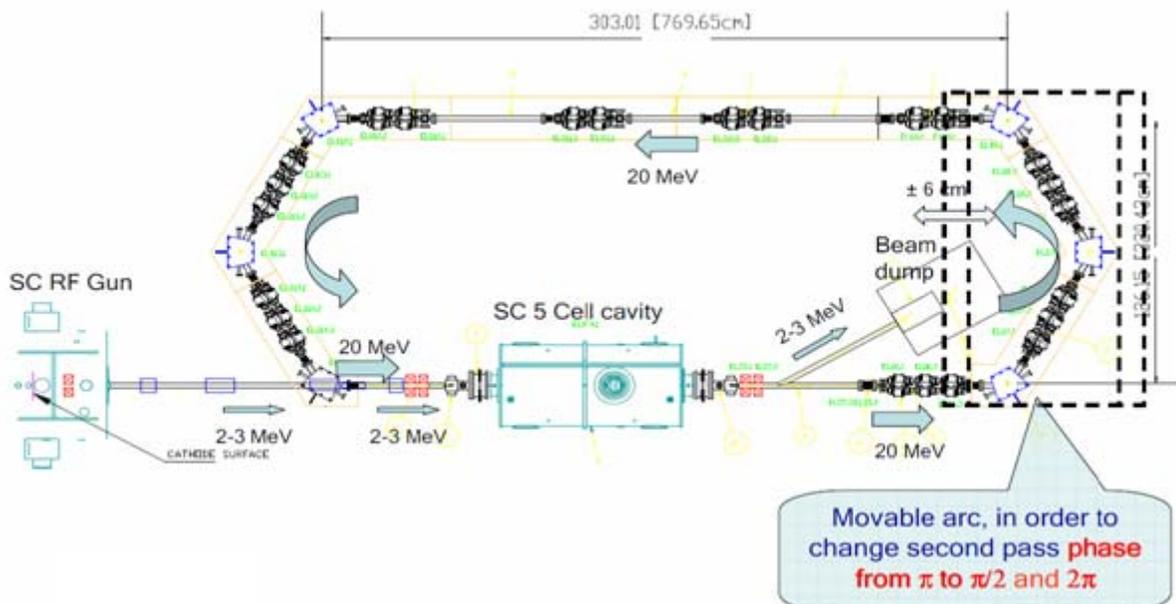
Figure 14: R&D ERL layout with indication of movable arc.
