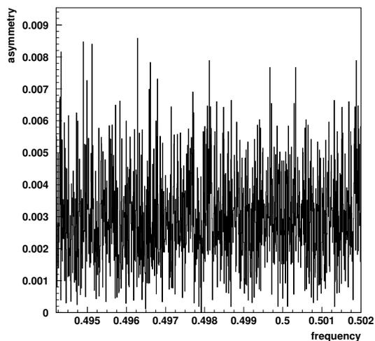
Figure 3.4: FFT amplitude of the asymmetry from polarimeter detectors 3 and 6. The FFT was applied to the first  $2^{19}$  turns after the injection event. The spin tune is expected to produce an amplitude at a frequency near 0.5. However, no definite signal can be seen here.
