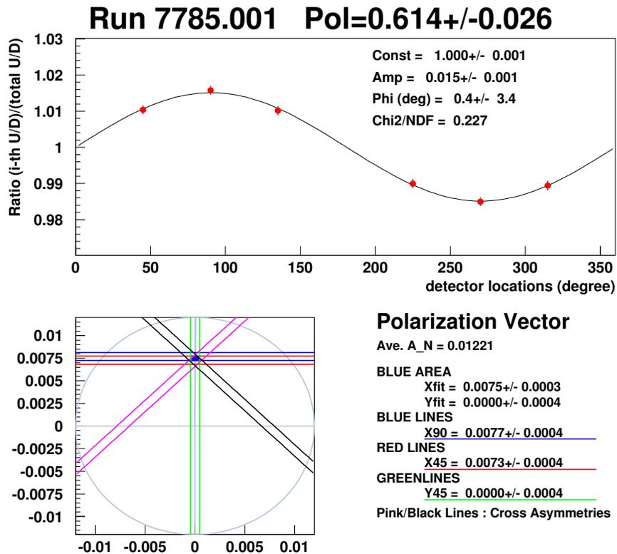
Figure 1.2: Example of the second page of the online plots display. At the top of the page, the polarimeter run number, the measured polarization, and statistical error are shown. This page shows plots of the ratio of spin up to spin down events vs. detector position and the measured polarization vector. In the lower-right corner, the average  $A_N$  and some measured asymmetries are displayed. Polarization is given by the “X fit” asymmetry divided by the average  $A_N$ .
