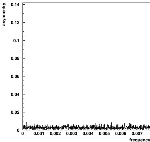
Figure 3.3: FFT amplitude of the asymmetry from polarimeter detectors 1 and 4. The asymmetry combines the data from two measurements. The FFT was applied to the first  $2^{19}$  turns after the injection event. A significant signal is observed at frequency 0. The amplitude is  $\sim 0.128$ . FFT analyses from later portions of the data show that this amplitude decreased over time, indicating depolarization of the beam.
