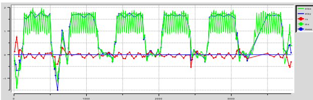
Figure 18: Yellow Horizontal Dispersion: Model (Green), Measured (Blue), and Residual (Red)
