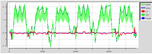
Figure 17: Blue Horizontal Dispersion with DHX angles correction: Model (Green), Measured (Blue), and Residual (Red)
