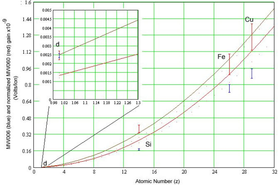
**Figure 2:** Data and fits for multiwire gain ( $V/lon$ ) vs.  $z$  for cases where  $\beta=0.43 \pm 0.01$  ( $d^{+1}$ ,  $Si^{+14}$  (charge +5 at MW006),  $Fe^{+26}$ , and  $Cu^{+29}$ ). This is a close-up of the graph in figure 1 for lower  $z$  including the deuteron case. The legend is the same as it is for figure 1.
