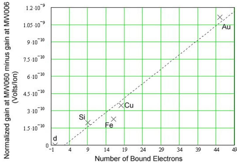
**Figure 3:** Normalized MW060 gain minus gain at MW006 ( $\Delta G$ ) versus number of bound electrons ( $N$ ) for ions at  $\beta=0.43$ . The dotted line is a linear fit of the data,  $\Delta G=(2.52e-11)N -(6.73e-11)$ .
