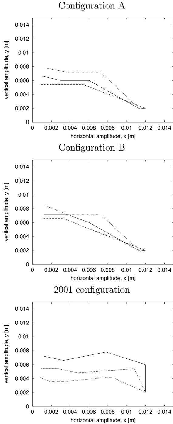
Figure 4: *Dynamic aperture just after the transition jump, for  $\Delta p/p = 0.0$  (solid), 0.002 (dashed) and  $-0.002$  (dotted), for  $\beta^* = 5$  m in all IPs. One  $\sigma$  corresponds to 0.6 mm in both planes for an emittance of  $\epsilon = 10\pi$  mm mrad. The top graph shows the situation with the jump sextupole configuration A, the middle one corresponds to configuration B, while the lower plot exhibits the dynamic aperture for the regular run 2001 scheme.*
