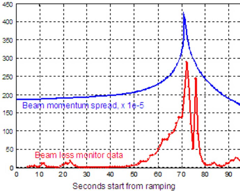
Figure 4: Beam loss at the loss monitor located at the 0.7 *cm* ridge, 39.4 *m* away from IP6. Ramp 6196, with 37 bunch mode,  $4.3 \times 10^9$  Cu ions per bunch, in a normal operation. RF voltage is 300 *kV* at the transition. The model beam momentum spread is shown for comparison. The beam loss is started 50 seconds after the ramping, 20 seconds before the transition.
