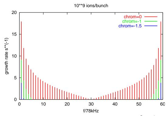
This shows the coupled bunch growth rates for 60 bunches and 10<sup>9</sup> ions/bunch for various chromaticities, as a function of observed frequency. The frequency dependence of the growth rate is due to the frequency dependence of the resistive wall impedance. Experimental tests should be fairly easy.
