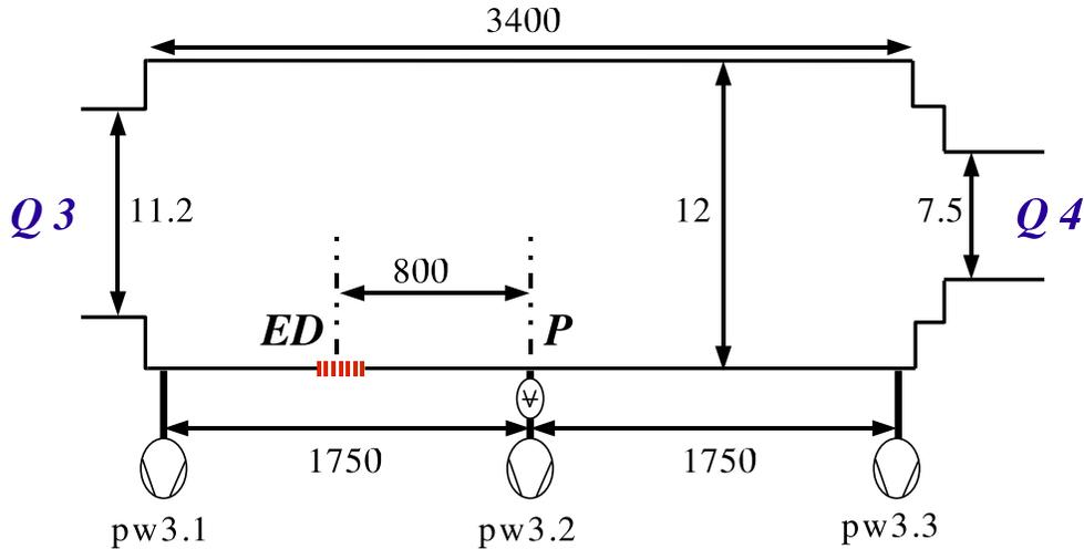
Figure 1: Geometry of the single beam pipe BO2, made of stainless steel and unbaked during Run-3. The electron detector location (marked with  $ED$ ) is about 8 m away from the pressure gauge and vacuum ion pump, whose location is marked with  $P$ . Distances are given in cm and are not to scale.
