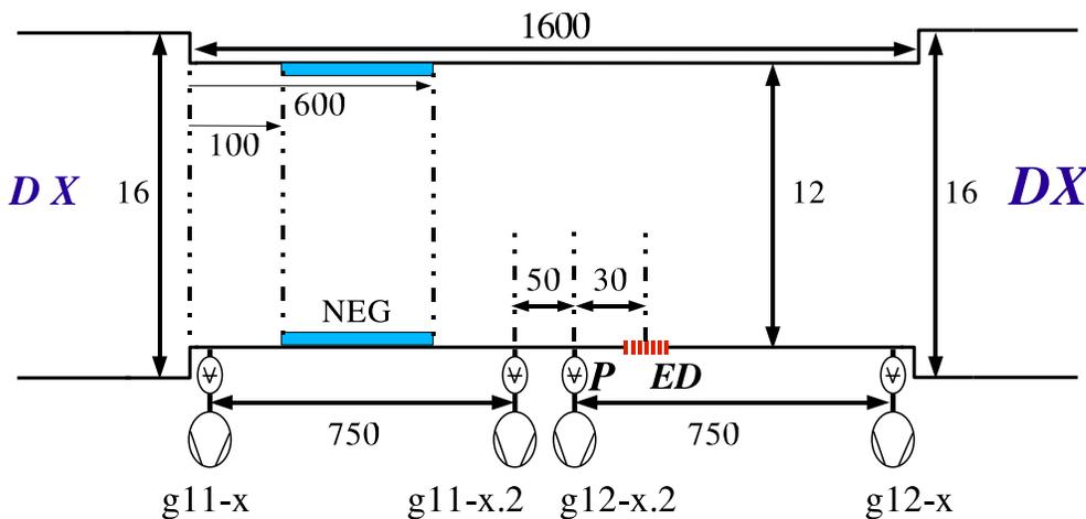
Figure 7: Geometry of the common beam pipe IR12, made of baked stainless steel. The electron detector location (marked with *ED*) is only 0.3 m away from the pressure gauge and vacuum ion pump, whose location is marked with *P*. Distances are given in cm and are not to scale.
