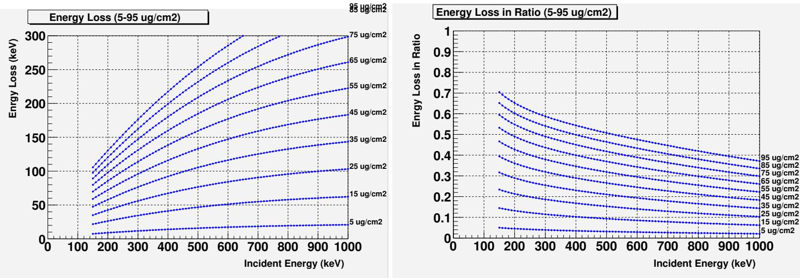
**FIGURE 6.** The left plot shows the energy loss,  $dE/dx$ , for different thickness dead layers, for carbon ions incident on silicon /citedEdx, vs. carbon energy. The right plot shows the fractional energy loss.
