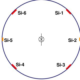
**FIGURE 3.** The layout of the silicon detectors inside the 15cm radius vacuum pipe of each RHIC polarimeter. The polarized proton beam direction is into the paper, and the carbon target is represented by the vertical line at the center of the vacuum pipe.
