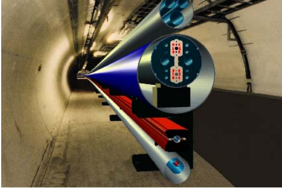
Figure 2: Cartoon drawing of the tunnel cross section in the VLHC collider arc, showing the low field ring with horizontally separated beams below the high field ring with vertically separated beams.
