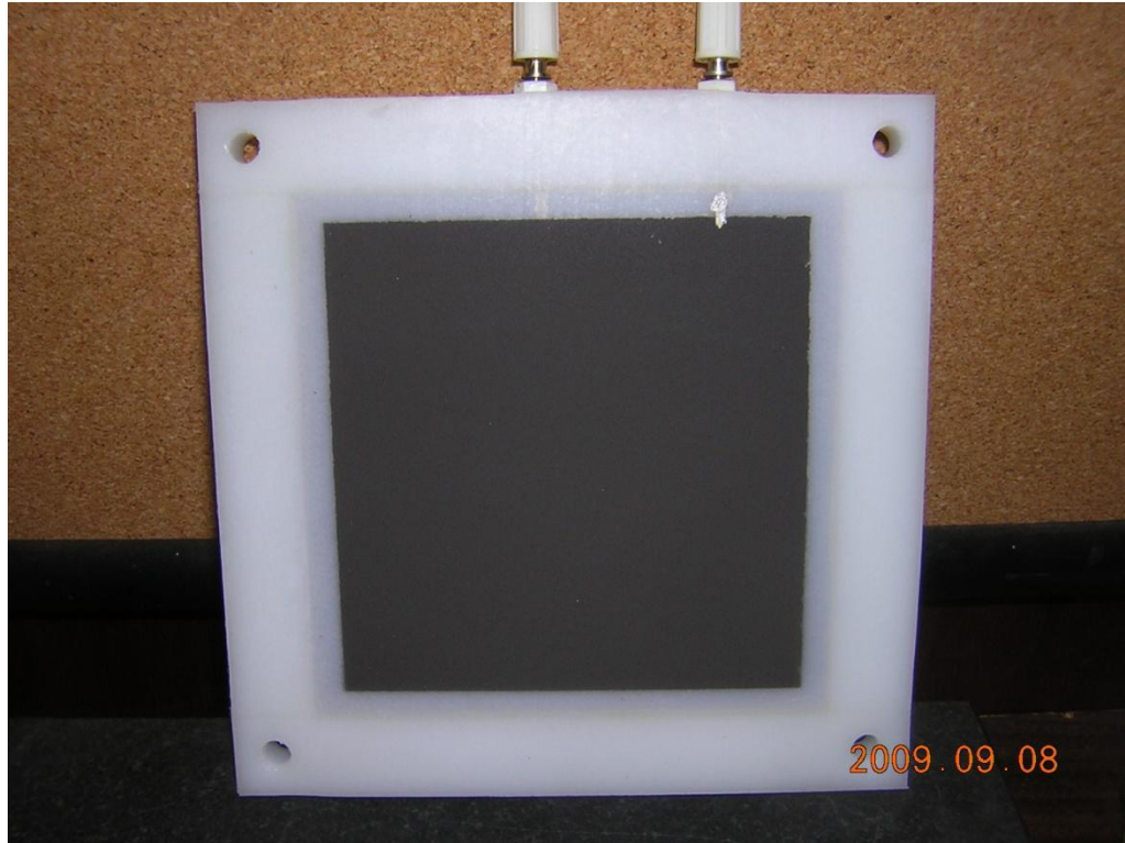
Figure 18: Signal chamber. Both sides are used for charge collection.
