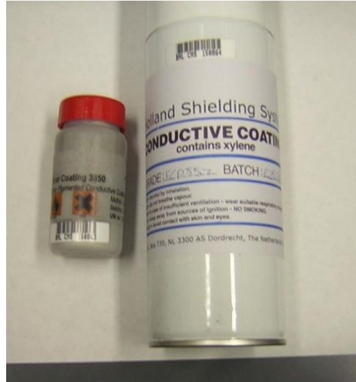
Figure 1: Aerosol spray paint and Silver Coating 3850.
