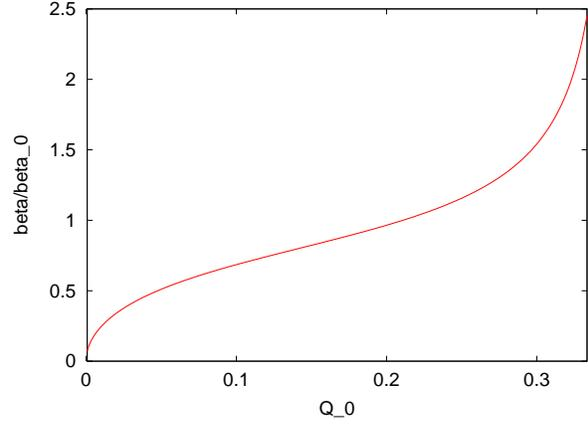
Figure 3: Dynamic  $\beta/\beta_0$  vs. base tune  $Q_0$  for a beam-beam parameter  $\xi = 0.08$ , calculated according to Equation (3).
