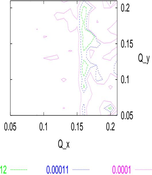
Figure 5: Contour plot of the horizontal rms electron beam size  $\sigma_x$  (in meters) vs. electron beam working point  $(Q_x, Q_y)$ .
