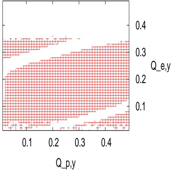
Figure 1: Tune diagram  $Q_{e,y}$  vs.  $Q_{p,y}$  in the vertical plane, for a beam-beam parameter of  $\xi = 0.08$ . The checkered areas indicate stable tune regions.
