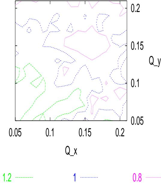
Figure 4: Contour plot of the resulting normalized luminosity  $\mathcal{L}/\mathcal{L}_0$  vs. horizontal and vertical electron beam tune.  $\mathcal{L}_0$  denotes the geometric design luminosity according to Table 1.
