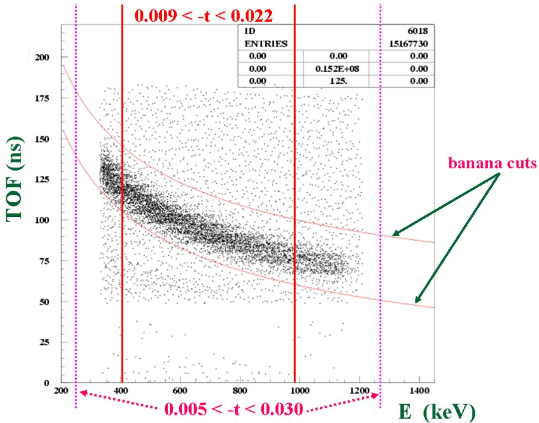
Figure 3: The banana curve (TOF versus Energy).
