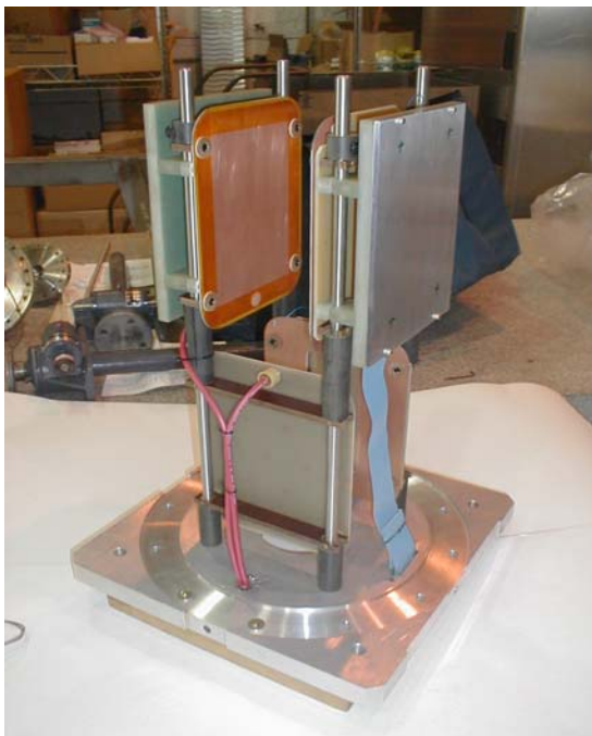
Figure 9: Photos of final assembly of EPM with permanent magnets
