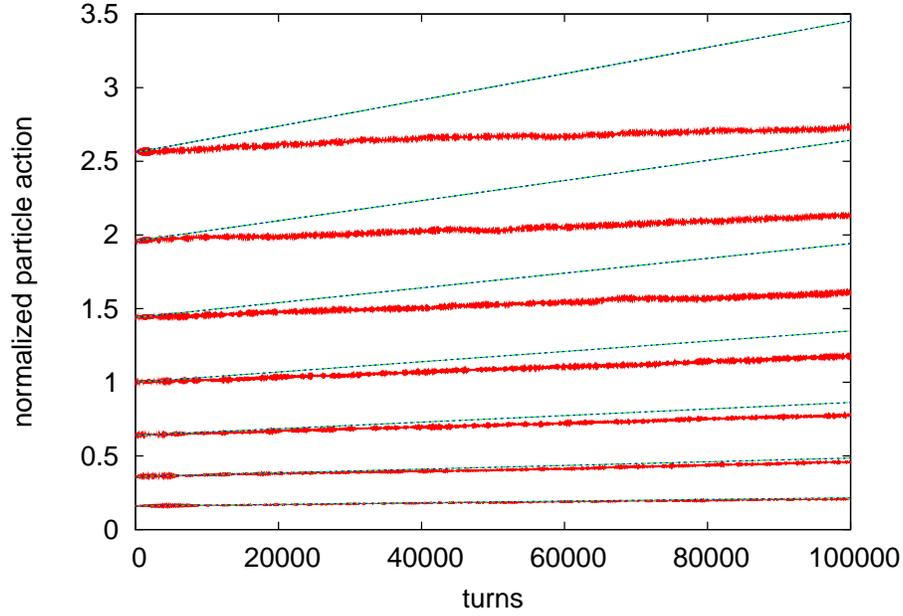
Figure 3: Normalized particle action  $J \cdot \beta / \sigma^2$  vs. turn number for different initial values of  $J$ . The red lines show simulated data for the nonlinear beam-beam force with fluctuating electron beam size  $\sigma_z$ . The magnitude of the fluctuation is set to  $\sqrt{\langle (\sigma_z^2 - \langle \sigma_z^2 \rangle)^2 \rangle} / \langle \sigma_z^2 \rangle = 0.03$ . The analytical result for the linearized beam-beam force is indicated by straight blue lines.
