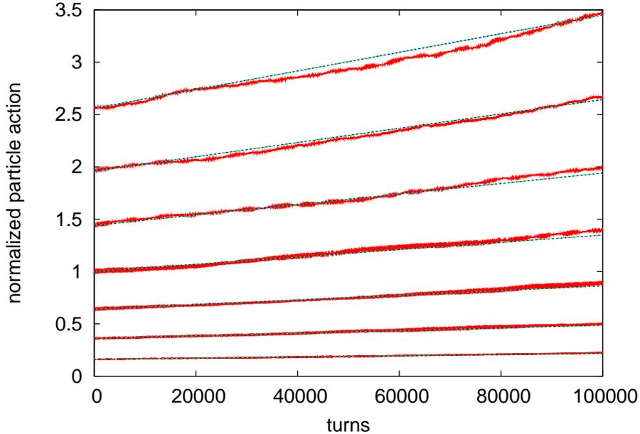
Figure 1: Normalized particle action  $J \cdot \beta/\sigma^2$  vs. turn number for different initial values of  $J$ , with the beam-beam force linearized according to Equation 3. The straight, blue lines correspond to the analytical result, Equation 9, while the red lines show simulated data.
