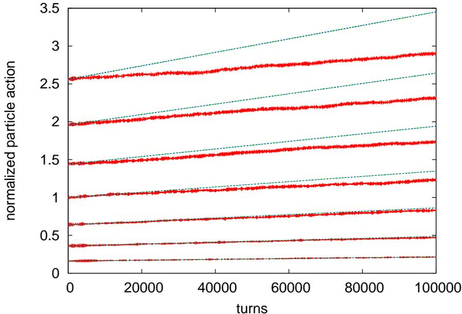
Figure 2: Normalized particle action  $J \cdot \beta / \sigma^2$  vs. turn number for different initial values of  $J$ . The analytical result for the linearized beam-beam force is indicated by blue lines, while the red lines show simulation data for the nonlinear beam-beam force with fluctuating electron beam intensity  $N_e$ . The rms width of the fluctuation is set to  $\sqrt{\langle (N_e - \langle N_e \rangle)^2 \rangle} / \langle N_e \rangle = 0.03$ .
