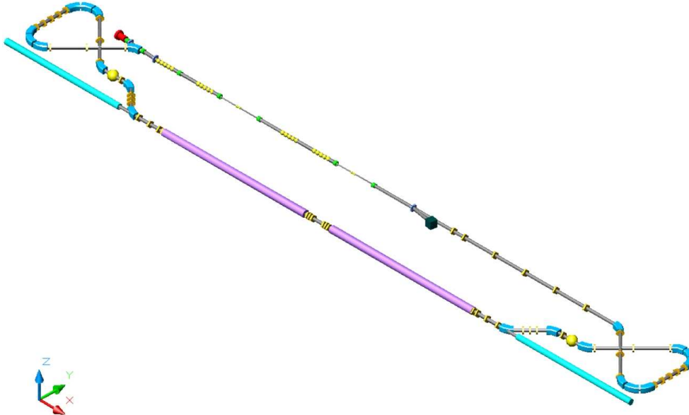
Figure 3.1: Schematic layout of the RHIC electron cooler (system shown for one ring). The photoinjector is shown in red, the superconducting energy-recovery linac is shown in yellow, the solenoid in purple and a section of the RHIC ring is shown in green.
