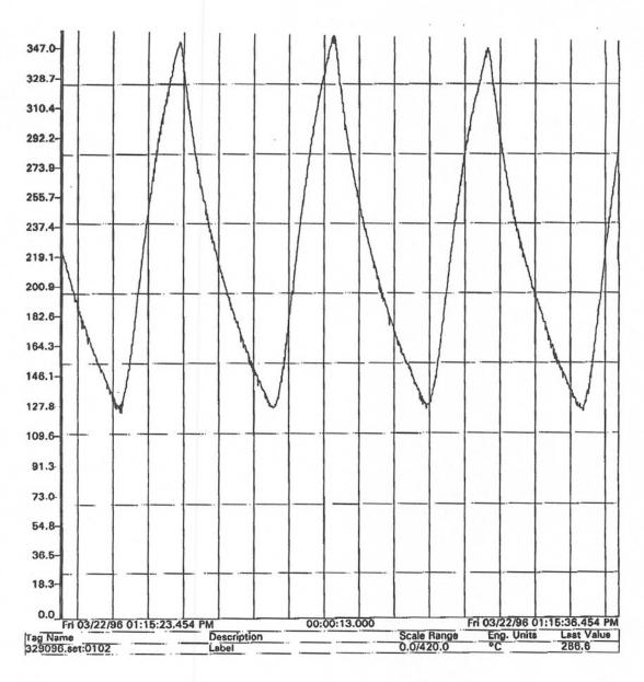
It must be noted that the spill of the AGS tends toward shortening on its own if left unattended by operators, and could shorten to as much as 0.5 seconds. If this should inadvertently occur during the spill, temperature in the target would rise and approximately double.
