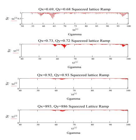
FIG. 5: Single particle tracking result through acceleration ramp at usual RHIC operating tunes with IP 6 and 8 squeezed to  $0.9~\mathrm{m}$  and remaining IP at  $5~\mathrm{m}$
