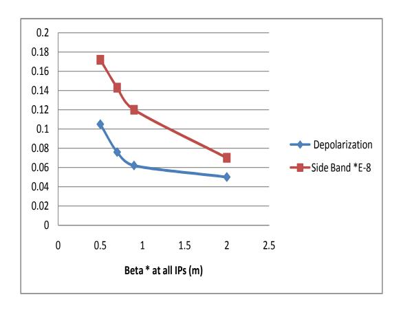
FIG. 4: Polarization response to beta star at 3rd order hybrid snake resonance
