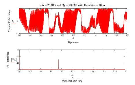
FIG. 1: 1st order hybrid snake resonance. Top plot vertical polarization. Bottom spin tune frequency: note 1st order resonance line at 0.315 and at 0.815 + 0.5 = 0.315.
