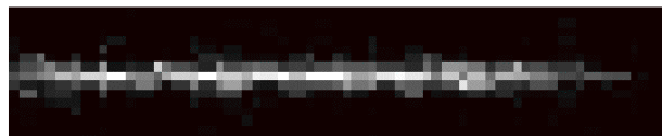
Fig. 12. A 1.7 mm thick slice through the activity distribution of the 3-D PET image. The beam entered from left. Horizontal (axial) dimension is 15.5 cm (full scanner FOV). Pixel size is 2.4 mm (H) by 1.7 mm (V).
