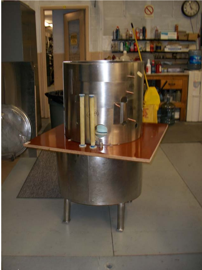
Fig. 3.4. Test cryostat with shield in place.
