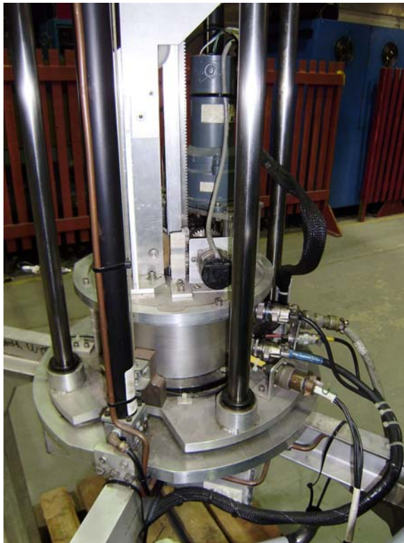
Figure 3.2. Close up vertical transporter drive mechanisms.
