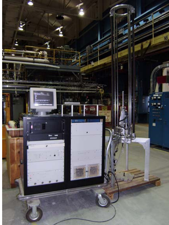
Figure 3.1. Vertical transporter and computer control cart.
