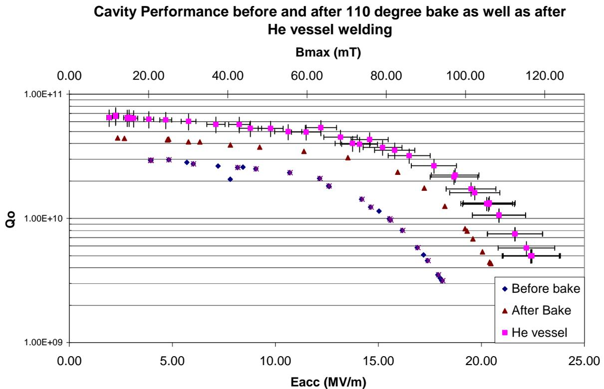
Figure 1. The plot of  $Q_o$  vs  $E_{acc}$  for three tests on the 5 cell cavity. The blue circles are before the 110 degree bake, the red triangles are after the 110 degree bake and the pink squares are with the He vessel attached.
