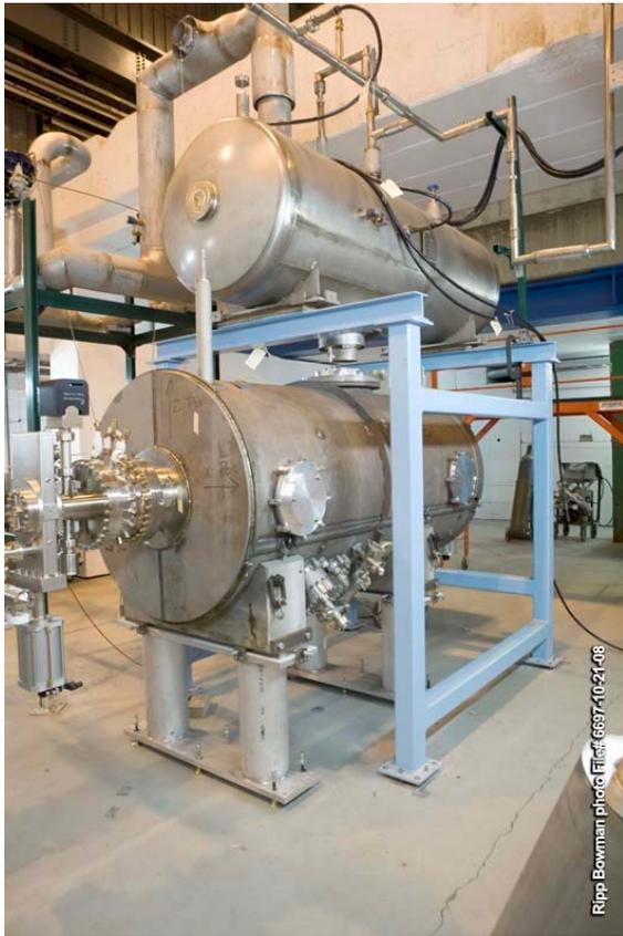
Figure 3. The cryomodule and liquid helium ballast tank installed in the ERL blockhouse.
