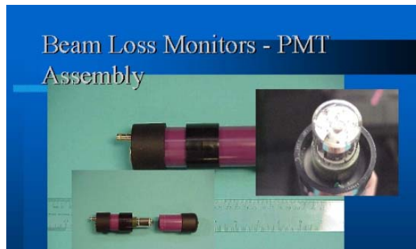
Fig. 14 PMT based BLM detector courtesy JLAB
