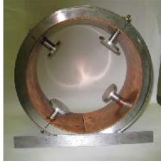
FIG. 17: Damper ring with four “mushroom” capacitive probes
