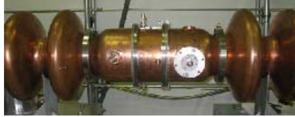
FIG. 16: Connecting tube with damper ring
