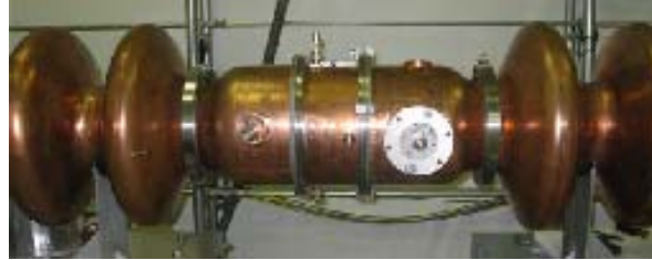
FIG. 16: Connecting tube with damper ring
