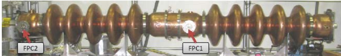
FIG. 10 : The HOM damper ring with capacitive probes between two copper cavities
