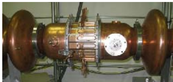
FIG. 21 : Ferrite HOM damper installed between the 5-cell Cu cavities
