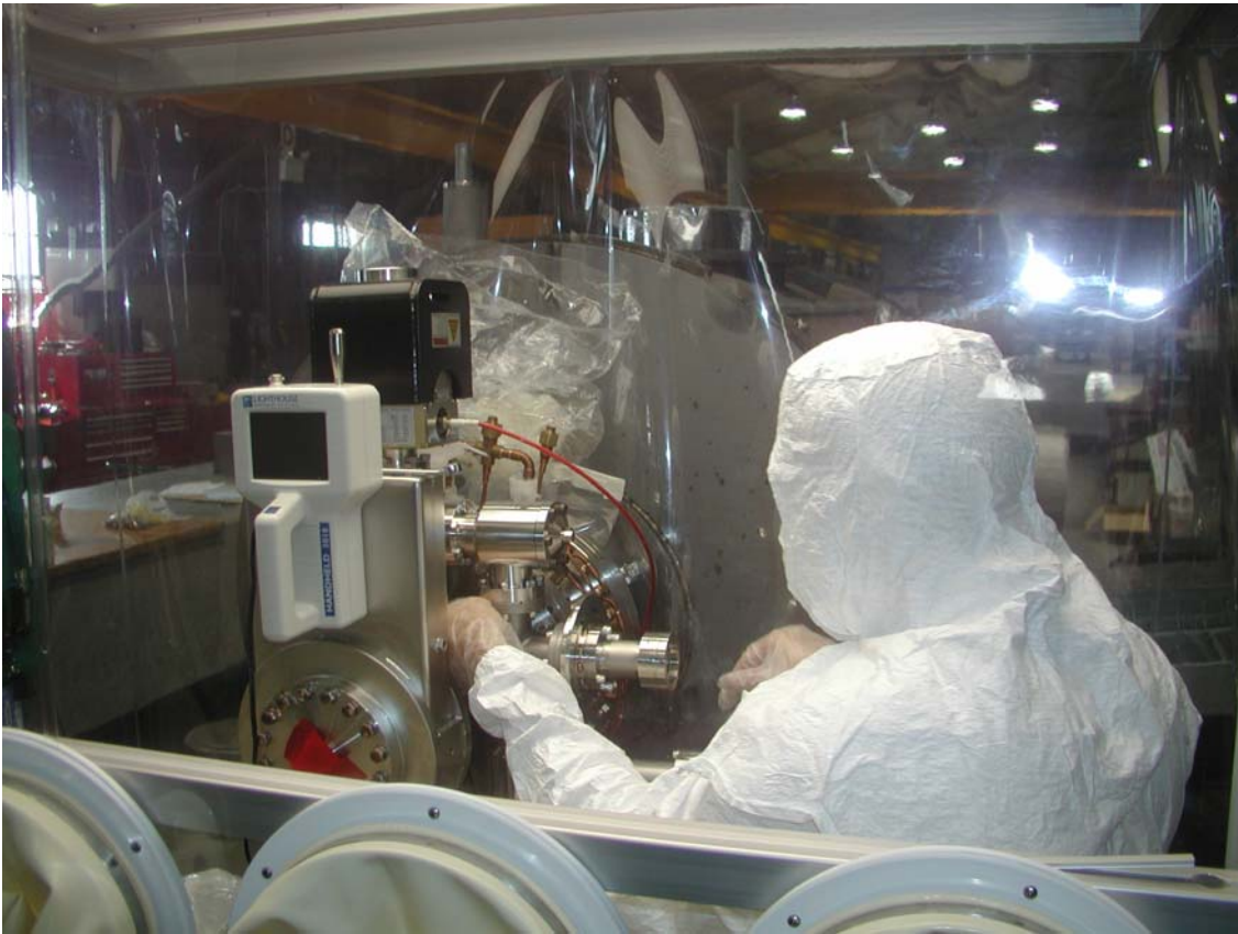
Figure 15. ERL Beamline Assembly Inside Portable Clean room
