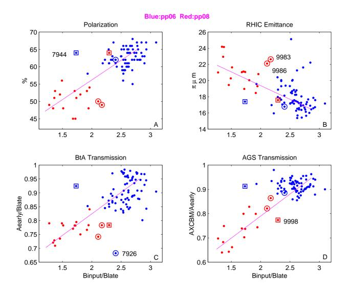
Figure 1: Booster scraping effects on RHIC beam polarization, RHIC beam emittance, and the BtA and AGS transmissions for pp06 and pp08 runs.
