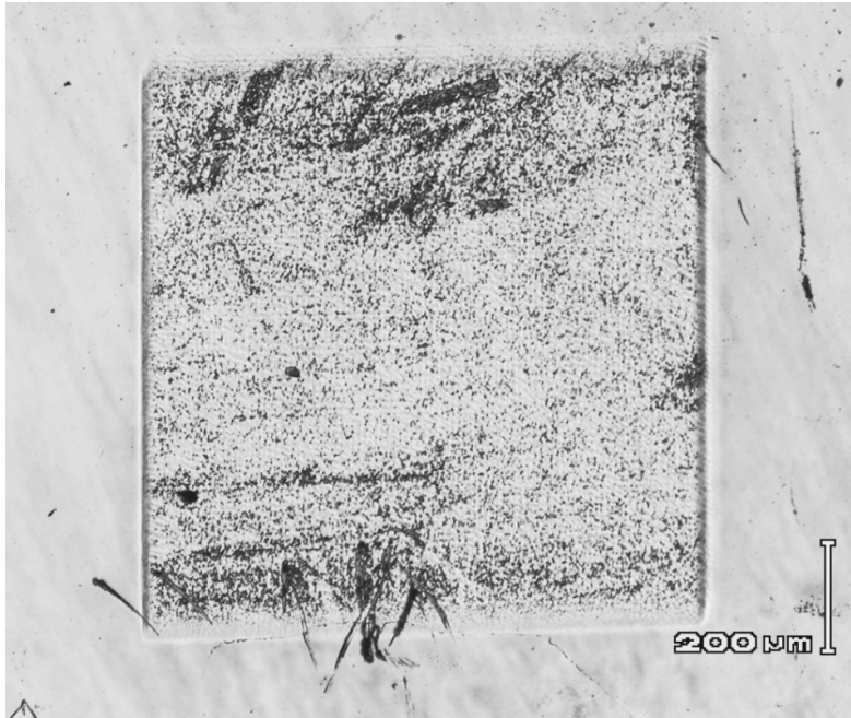
Figure 4.11: Optical microscope picture of 213nm laser ablated single crystal diamond. (This picture is taken by J. Smedley and T. Rao)
