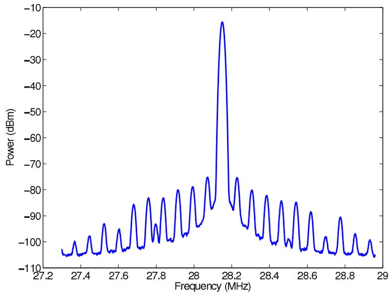
Figure 3: Blue ring spectrum near the fundamental mode of the 28 MHz cavity.
