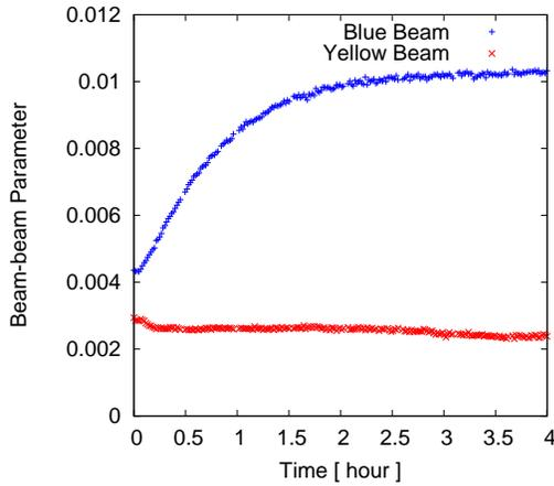
Figure 5: Calculated beam-beam parameters for fill 16911.
