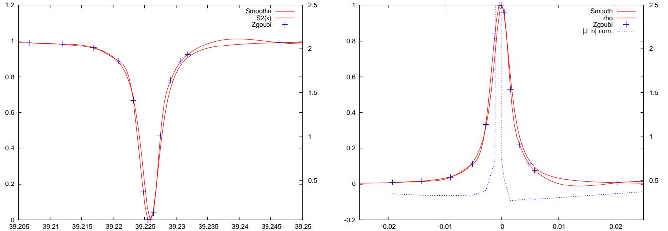
Figure 144: Matching  $S_z^2(\Delta)$  (left, Eq. 4) and  $\rho^2(\Delta)$  (right, Eq. 5) The right plot also shows  $|J_n|^2$  from numerical data (with expectable lack of accuracy in the region  $\Delta \rightarrow 0$ ).
