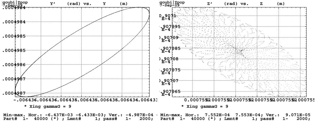
Figure 160: The particle sits on H and V closed orbits - observed at 'Begin SUPERA' (entrance to A1BF main dipole). Namely, the particle describes quasi zero  $\epsilon_x$  and  $\epsilon_y$  invariants, as shown here.
