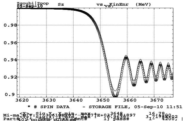
Figure 156: Superimposition of Fresnel integral model (squares) and zgoubi tracking (solid line) in a case of greater effect compared to the previous Fig. 155 :  $\epsilon_z/\pi = 0.01 \cdot 10^{-6}$ . The truncation of Froissard-Stora formula leads to an overestimate of  $p_f/p_i$  (Eq. 7).
