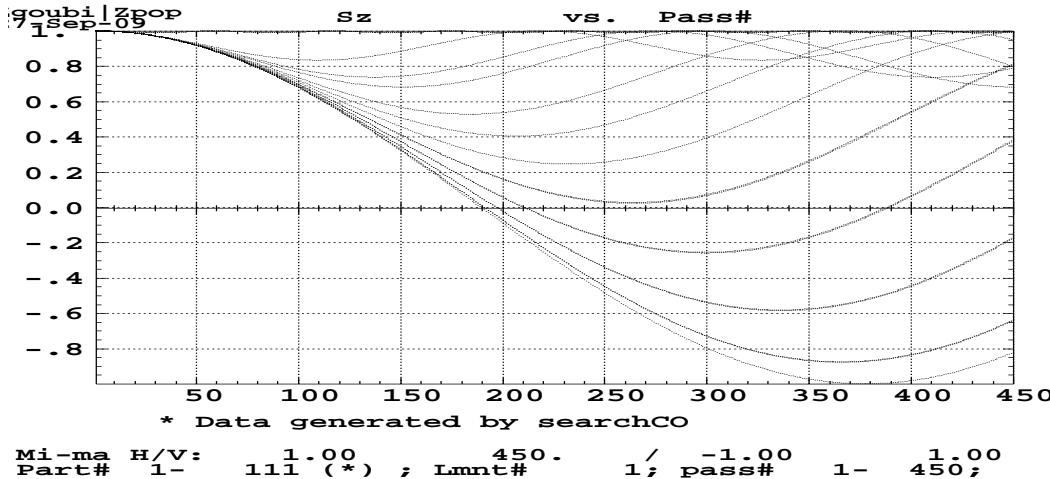
Figure 140:  $S_z$  versus turn number for various distances to the resonance.
