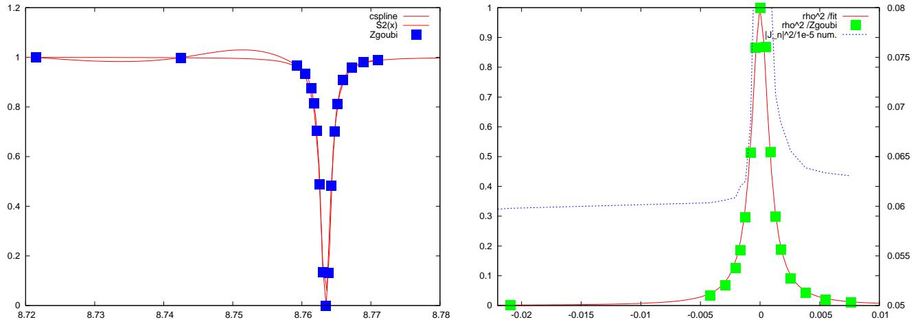
Figure 138: Matching  $S_z^2(\Delta)$  (left, Eq. 4) and  $\rho^2(\Delta)$  (right, Eq. 5) The right plot also shows  $|J_n|^2$  from numerical data (with expectable lack of accuracy in the region  $\Delta \rightarrow 0$ ).
