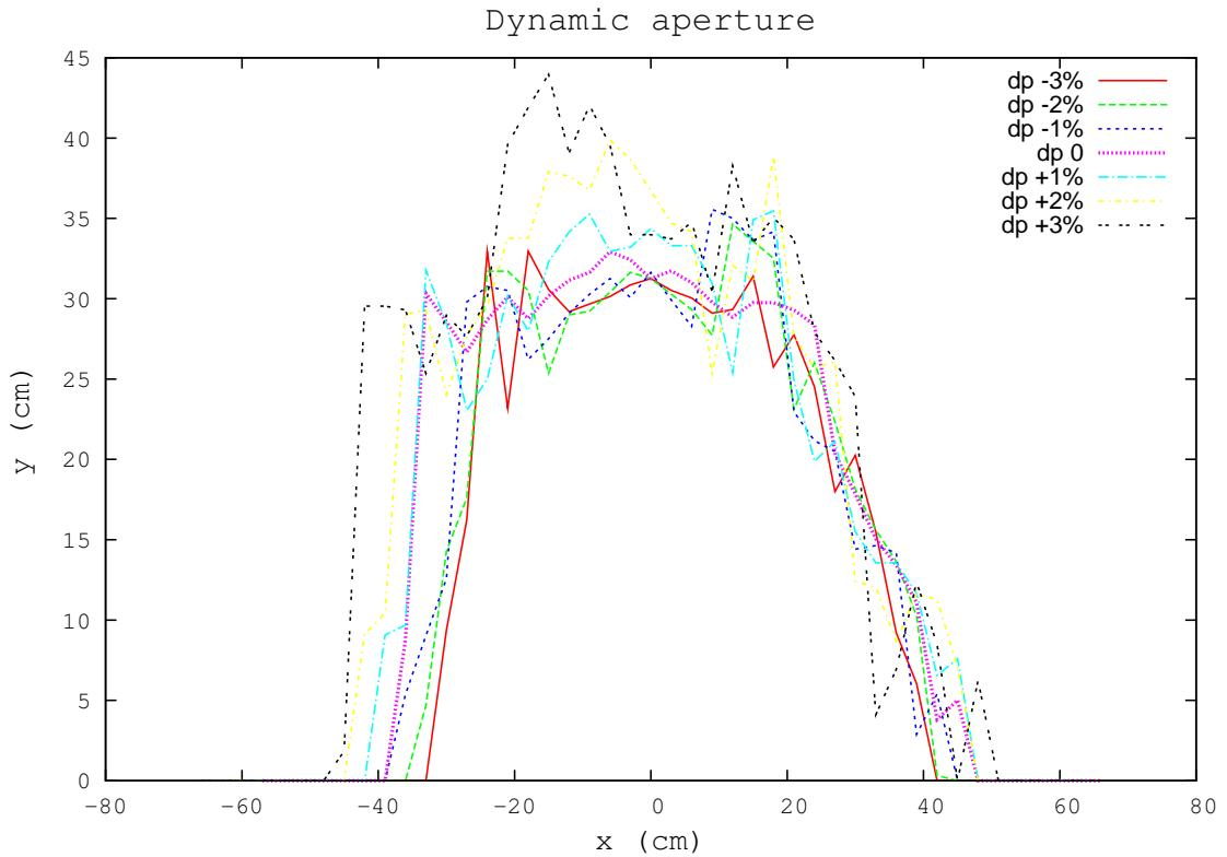
Figure 8: Dynamical apertures at  $\delta p/p = 0, \pm 1, \pm 2, \pm 3\%$ . 3 cm step in  $x$ , 2 mm precision on 1000-turn maximum vertical stable amplitude.
