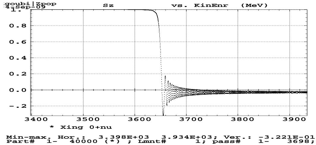
Figure 25:  $S_z$  versus kinetic energy, 7 particles evenly spread on  $\epsilon_z/\pi = 0.2$  mm.mrad invariant.
