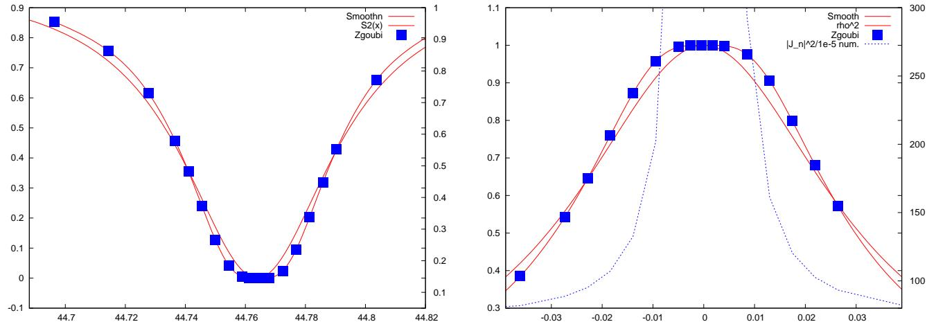
Figure 153: Matching  $S_z^2(\Delta)$  (left, Eq. 4) and  $\rho^2(\Delta)$  (right, Eq. 5) The right plot also shows  $|J_n|^2$  from numerical data (with expectable lack of accuracy in the region  $\Delta \rightarrow 0$ ).
