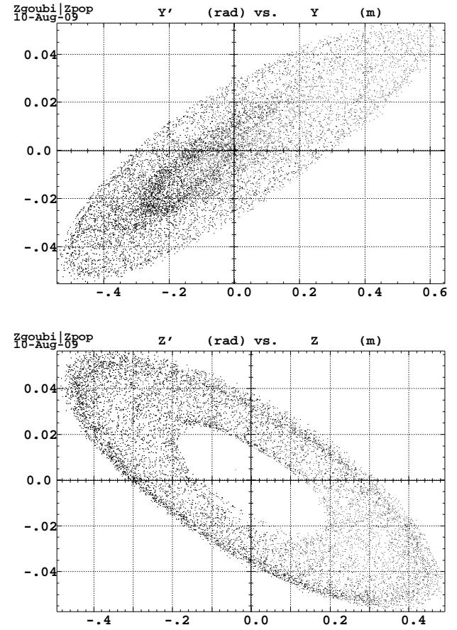
Figure 6: Maximum vertical stable amplitude, 1000 turns, showing H-V emittance exchange,  $\delta p/p = 0$ . Top plot : coupling induced  $x$ -motion ; bottom plot : vertical donut at maximum stable amplitude. Hard edge optical elements.
