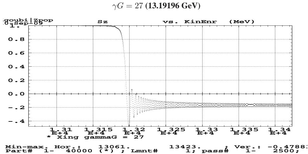
Figure 123:  $S_z$  versus kinetic energy. Check : 36-Qy next to  $gG=27$  is on the path at  $E=13.31575$  GeV, yet not visible as expected since  $\epsilon_z \approx 0$ .
