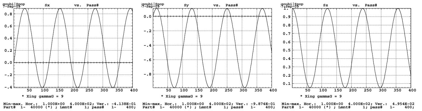
Figure 161: From top to bottom,  $S_x$   $S_y$   $S_z$  versus turn number observed at 'Begin SUPERA'. Static case ( $T = 3775.00$  GeV), given  $\vec{S}_{\text{initial}} = \vec{S}_z$ .
