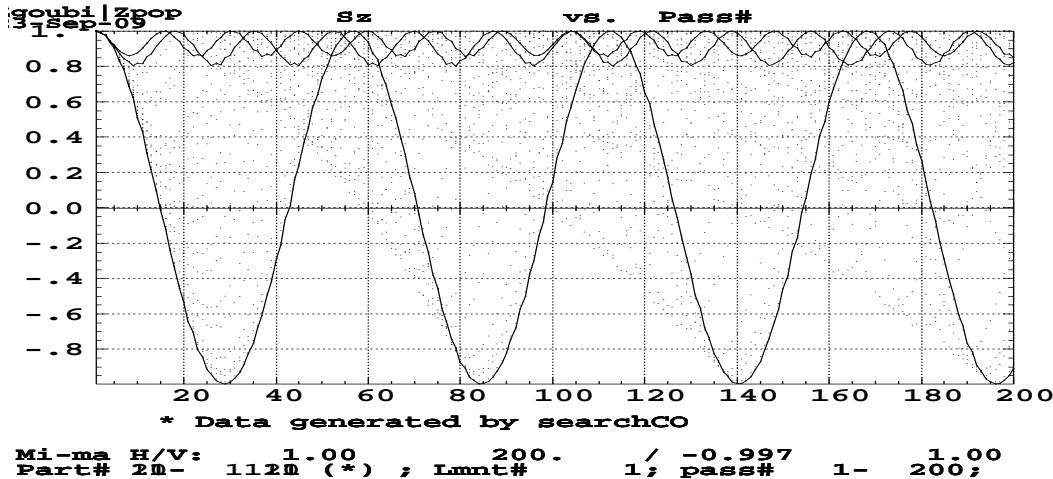
Figure 152:  $S_z$  versus turn number for various distances to the resonance.
