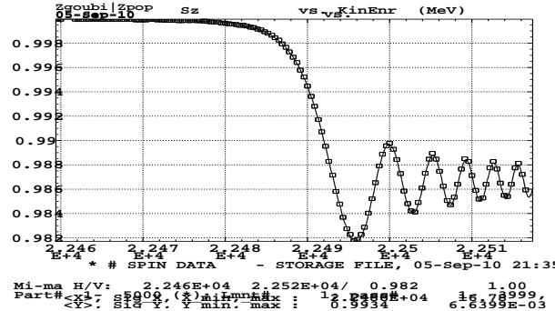
Figure 157: Superimposition of Fresnel integral model (squares) and zgoubi tracking (solid line)  $\epsilon_z/\pi = 0.0001 10^{-6}$ .
