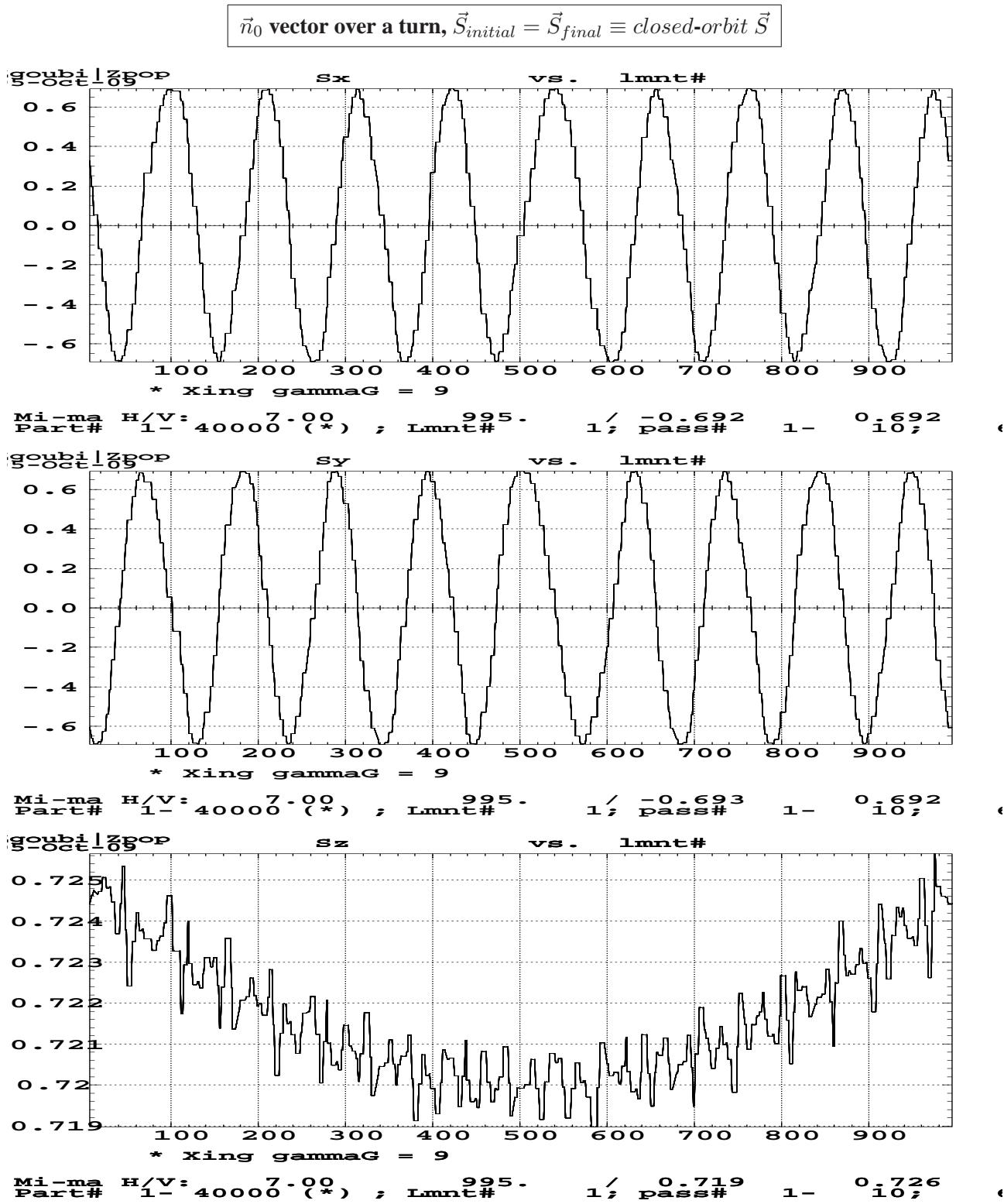
Figure 162: From top to bottom,  $S_x$   $S_y$   $S_z$  along machine circumference versus pick-up number (about 990 P-US over the 807 m circumference). Static case ( $T = 3775.00$  GeV), given  $\vec{S}_{initial} = \vec{S}_{final} \equiv$  closed-orbit  $\vec{S}$ .
