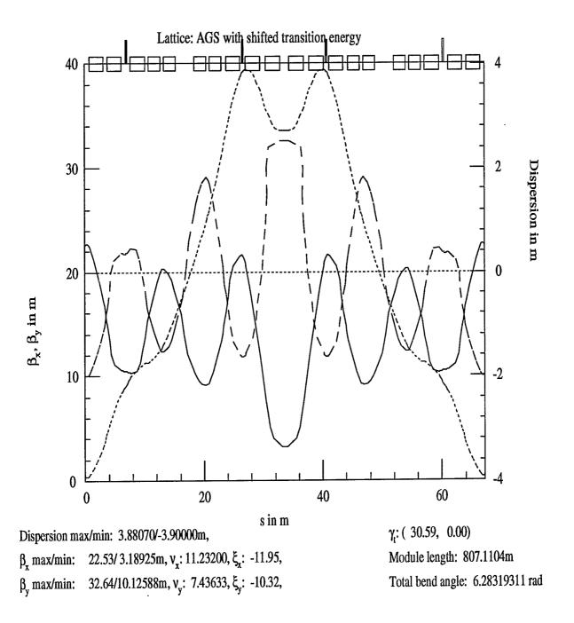
Figure 2: Orbit Functions in AGS lattice with shifted magnets and quads
