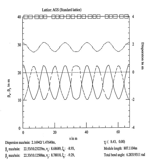
Figure 1: Orbit Functions in standard AGS Lattice
