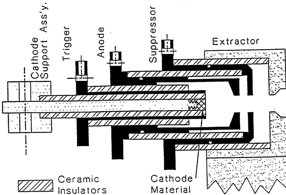
Figure 2. Schematic of a micro-MEVVA, which was fabricated and operated at BNL [12].
