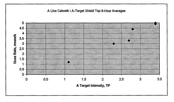
Survey Instrument Measurements
