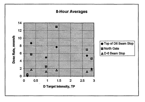
The dose rates in and around the D Line could not be related in any discernible way to intensity changes on the D target. The D target was minimally used during most of the study period. Changes in dose rates along the D Line may have been influenced by water pipes filled with water from other beam lines. They may also have been influenced by radiation levels in the AGS Ring which is proximate to D Line.
