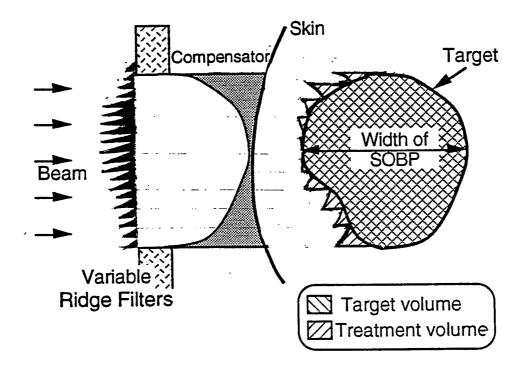
Figure 2. Variable range modulation scheme.
