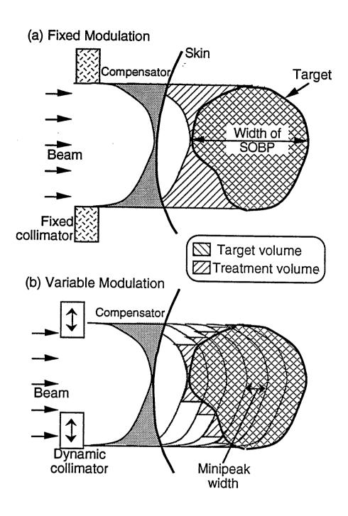
Figure 1a. Fixed energy modulation scheme.
