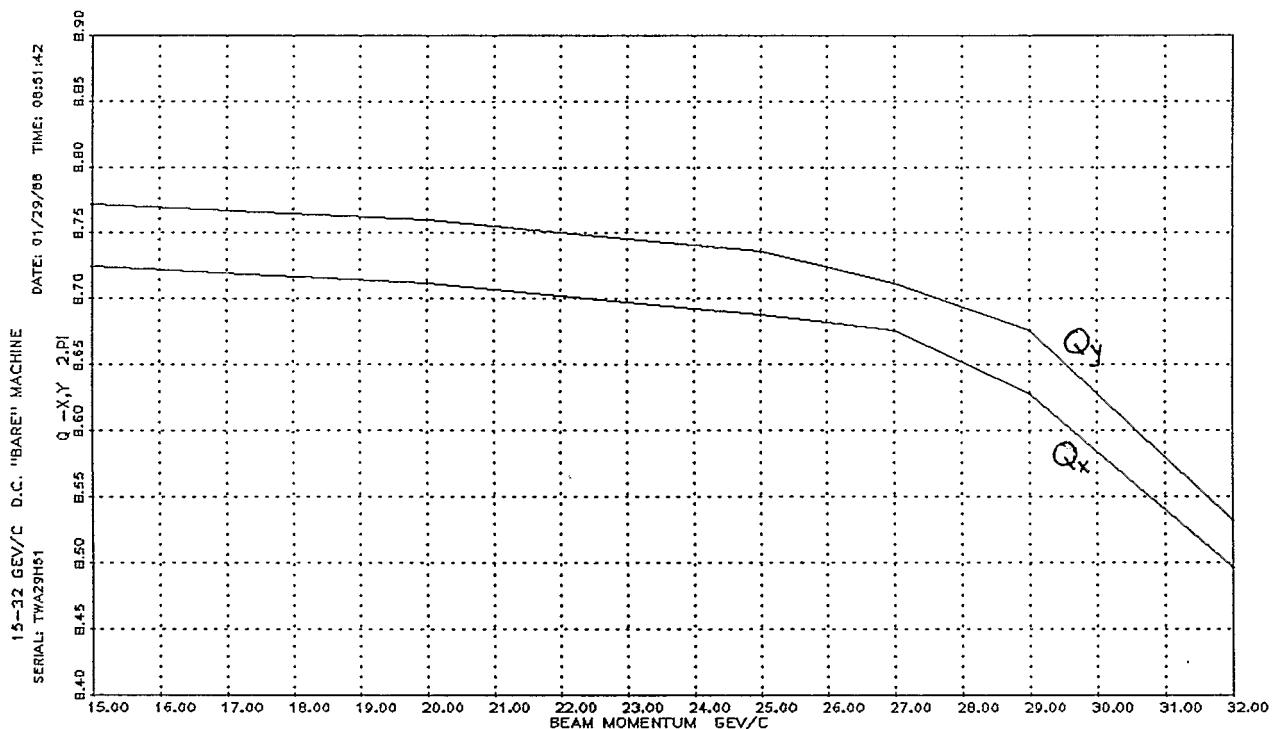
Figure 25. Energy Dependence of the Horizontal Tune,  $Q_x$ , and Vertical Tune,  $Q_y$ , for the D.C. "Bare" Machine (main magnets only) at high fields: 15-32 GeV/c. (Corresponds to Figure 5.) These tunes are exactly 12 times the respective values of  $M_u$  at the end of one superperiod.
