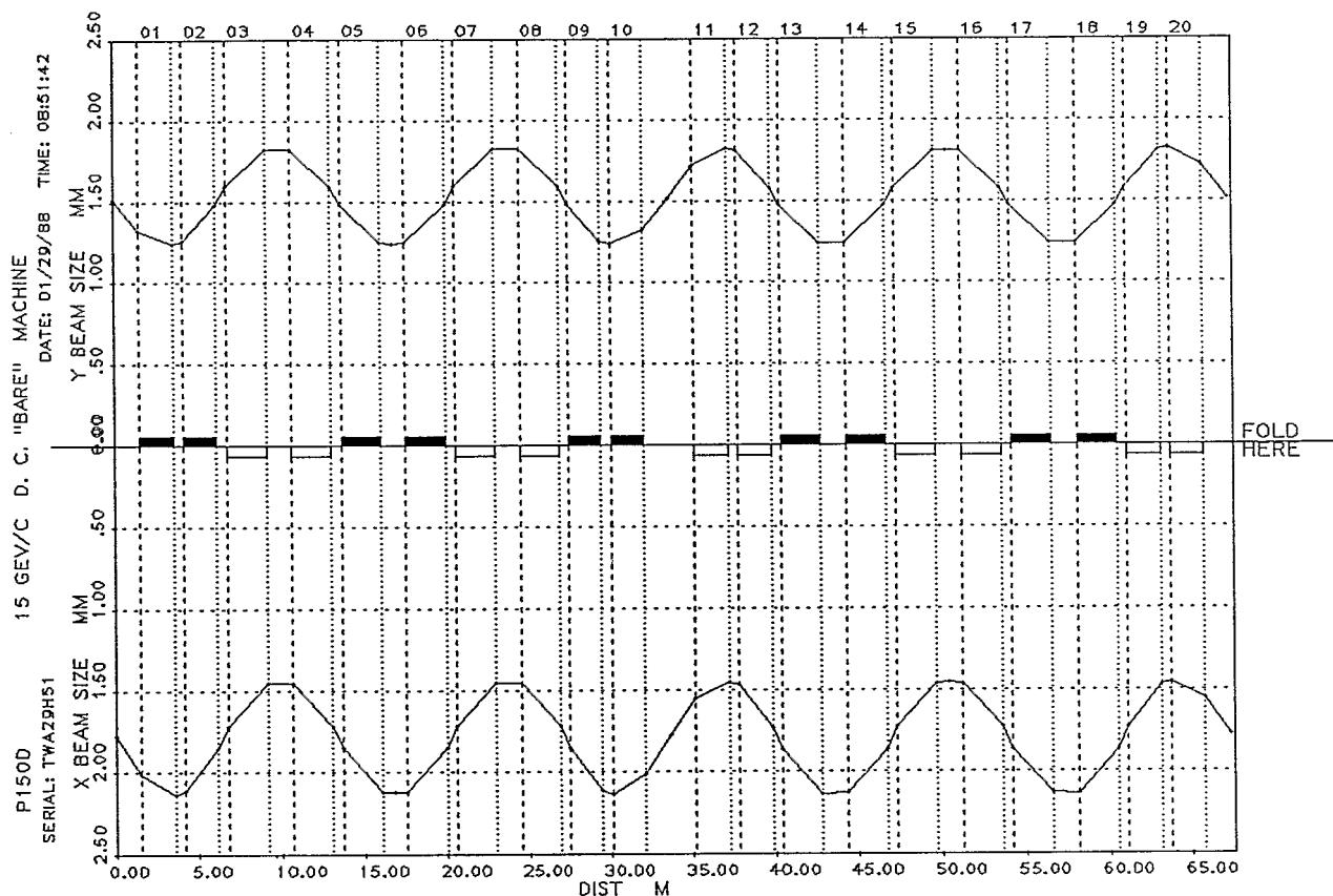
Figure 35. Beam Sizes (in mm) of the D. C. "Bare" Machine at 15 GeV/c, given for one superperiod. The y-direction (with scale increasing upward) appears in the upper half of the panel, while the x-direction (with scale increasing downward) is shown in the lower half of the panel.
