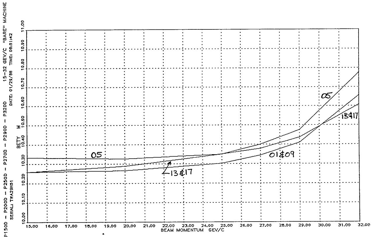
Figure 22. Energy Dependence of the Minima in Beta-y (in meters) for the D. C. "Bare" Machine (main magnets only) at high fields: 15-32 GeV/c. (Corresponds to Figure 2.) The several minima are labelled by the machine section in which they occur.
