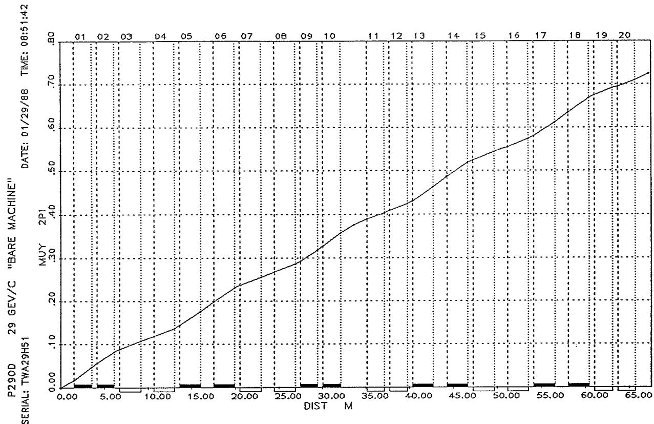
Figure 17. Phase Function  $\text{Mu-y}$  (in units of  $2\pi$  radians) for the D. C. "Bare" Machine (main magnets only) at 29 GeV/c, given for one superperiod.
