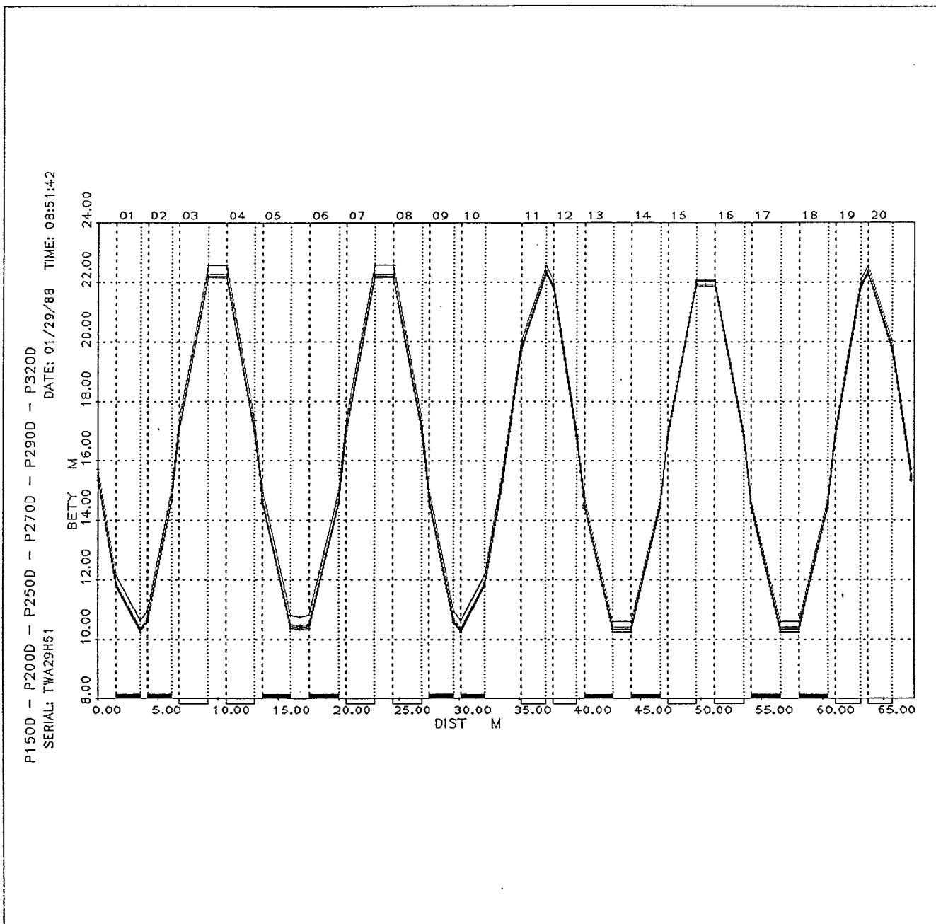
Figure 2. Courant-Snyder Parameter Beta-y (in meters) for the D.C. "Bare" Machine (main magnets only) at high fields: 15-32 GeV/c, given for one superperiod.
