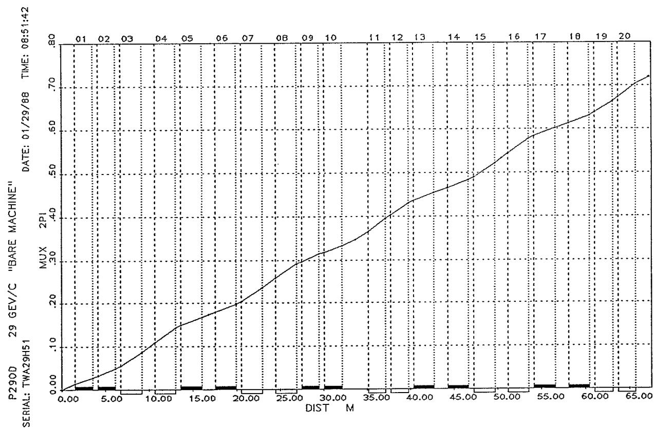
Figure 16. Phase Function Mu-x (in units of  $2\pi$  radians) for the D. C. "Bare" Machine (main magnets only) at 29 GeV/c, given for one superperiod.
