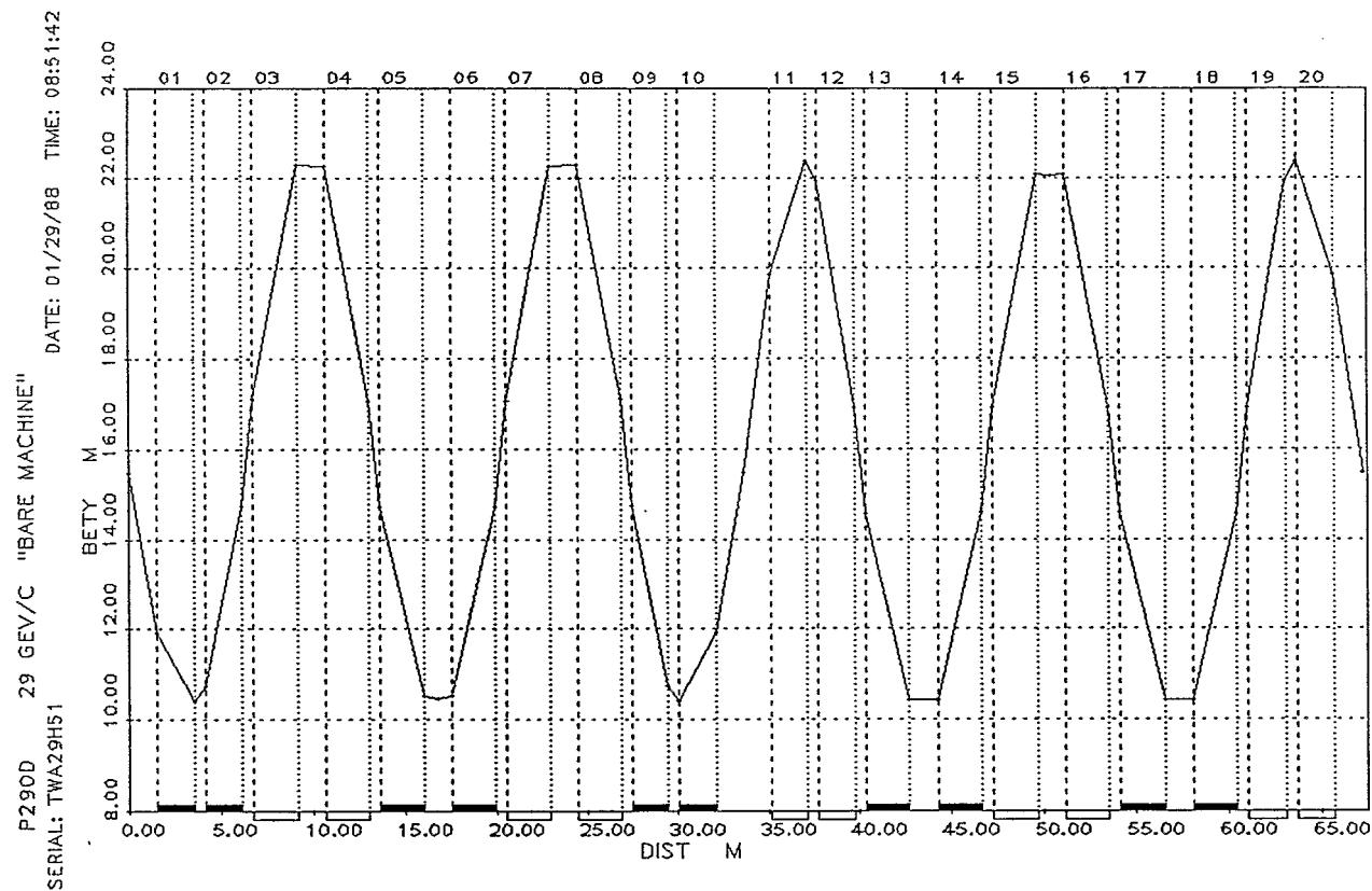
Figure 15. Courant-Snyder Parameter Beta-y (in meters) for the D. C. "Bare" Machine (main magnets only) at 29 GeV/c, given for one superperiod.
