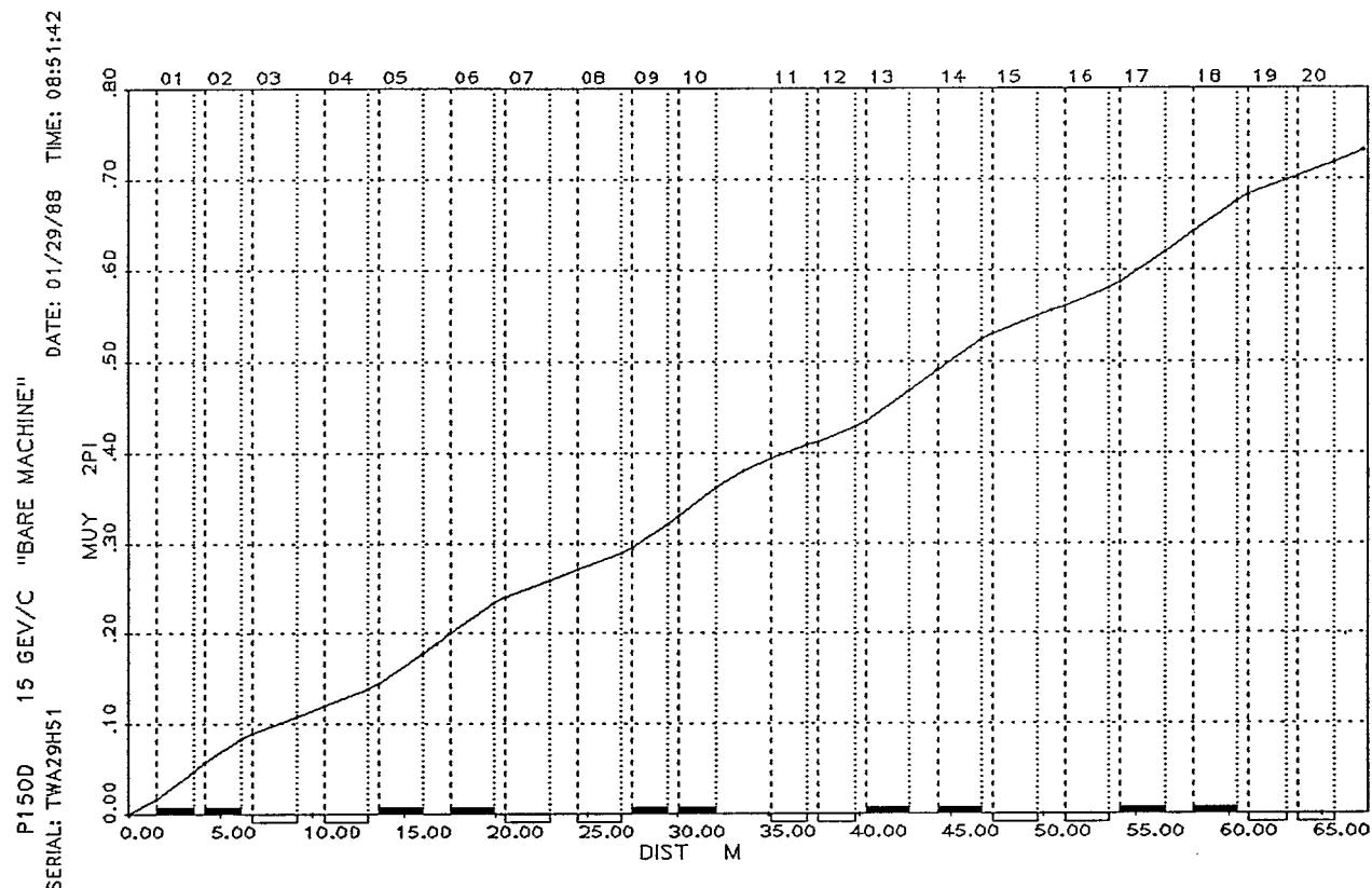
Figure 12. Phase Function  $\mu_y$  (in units of  $2\pi$  radians) for the D. C. "Bare" Machine (main magnets only) at 15 GeV/c, given for one superperiod.
