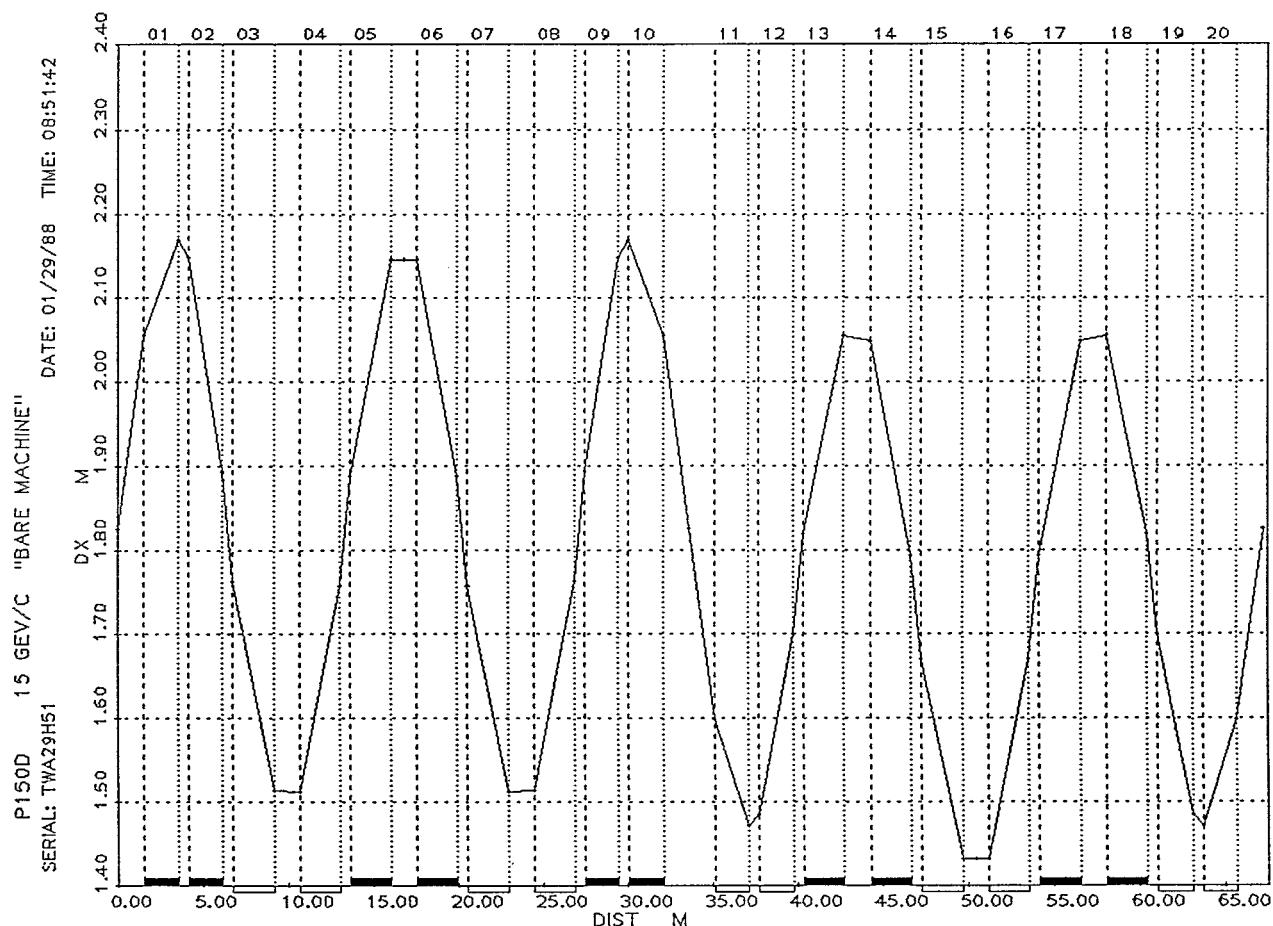
Figure 13. Dispersion Function  $dx$  (in meters) for the D. C. "Bare" Machine (main magnets only) at 15 GeV/c, given for one superperiod.
