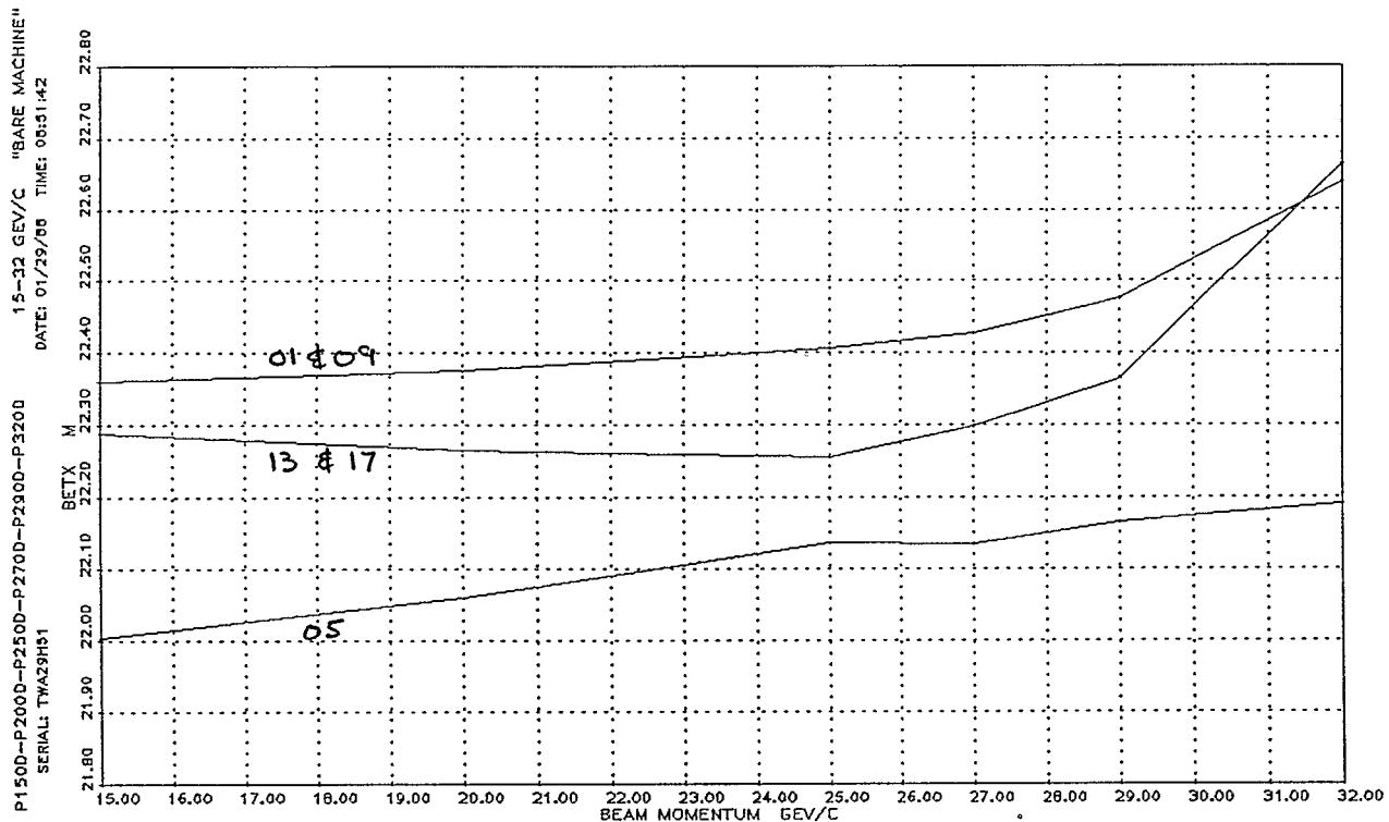
Figure 19. Energy Dependence of the Maxima in Beta-x (in meters) for the D. C. "Bare" Machine (main magnets only) at high fields: 15-32 GeV/c. (Corresponds to Figure 1.) The several maxima are labelled by the machine section in which they occur.
