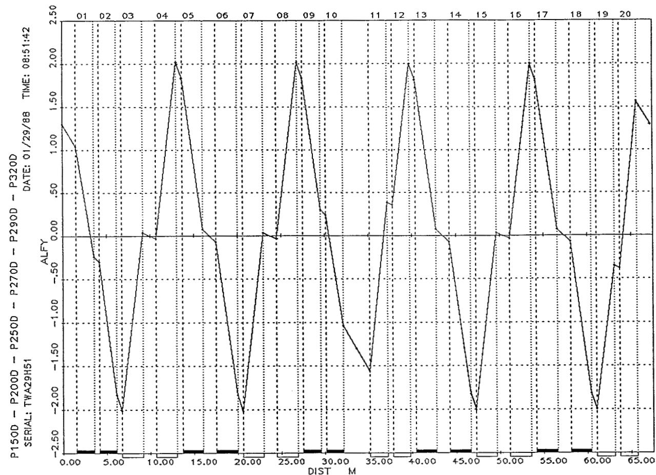
Figure 4. Courant-Snyder Parameter Alpha-y (dimensionless) for the D. C. "Bare" Machine (main magnets only) at high fields: 15-32 GeV/c, given for one superperiod.
