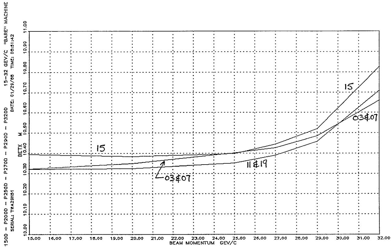
Figure 20. Energy Dependence of the Minima in Beta-x (in meters) for the D. C. "Bare" Machine (main magnets only) at high fields: 15-32 GeV/c. (Corresponds to Figure 1.) The several minima are labelled by the machine section in which they occur.
