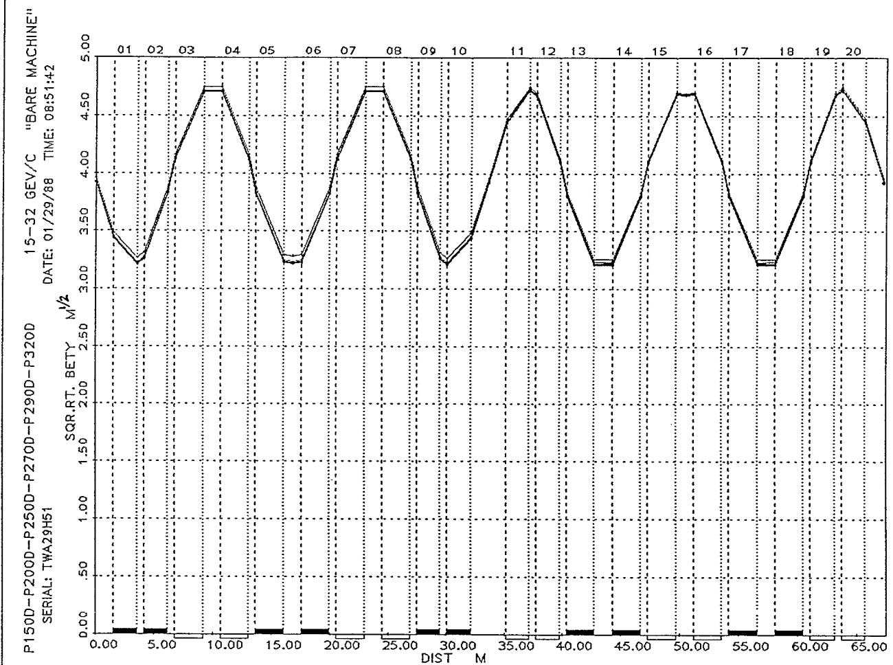
Figure 34. Courant-Snyder Parameter Beta-y shown on a square root scale for the D.C. "Bare" Machine (main magnets only) at high fields: 15-32 GeV/c, given for one superperiod. (Corresponds to Figure 2 which has a linear scale.)
