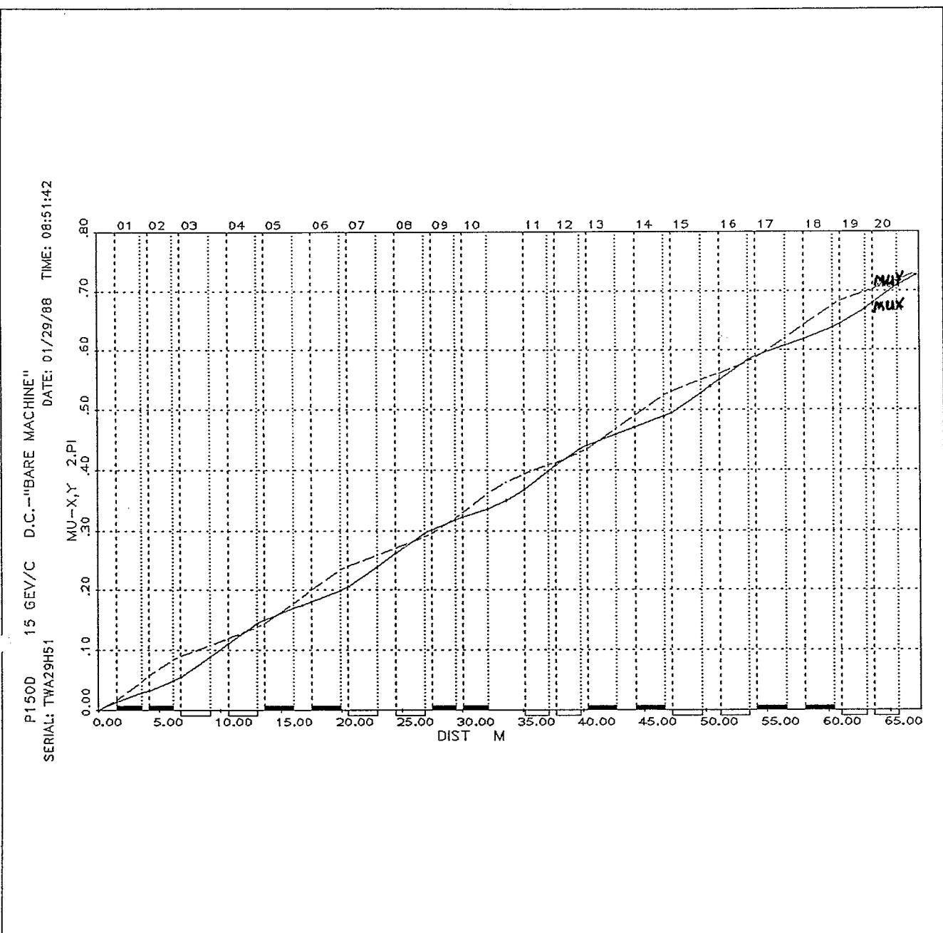
Figure 29. Phase Functions  $\text{Mu}-x$  and  $\text{Mu}-y$  (in units of  $2\pi$  radians) for the D.C."Bare" Machine (main magnets only) at 15 Gev/c, shown on the same plot. Note that only phase advance is meaningful. A different choice of zero-point would result in an upward or downward displacement of  $\text{Mu}-x$  relative to  $\text{Mu}-y$ .
