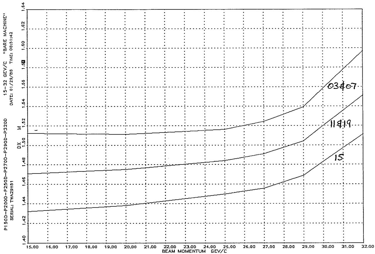
Figure 24. Energy Dependence of the Minima in Dispersion (in meters) for the D. C. "Bare" Machine (main magnets only) at high fields: 15-32 GeV/c. (Corresponds to Figure 7.) The several minima are labelled by the machine section in which they occur.
