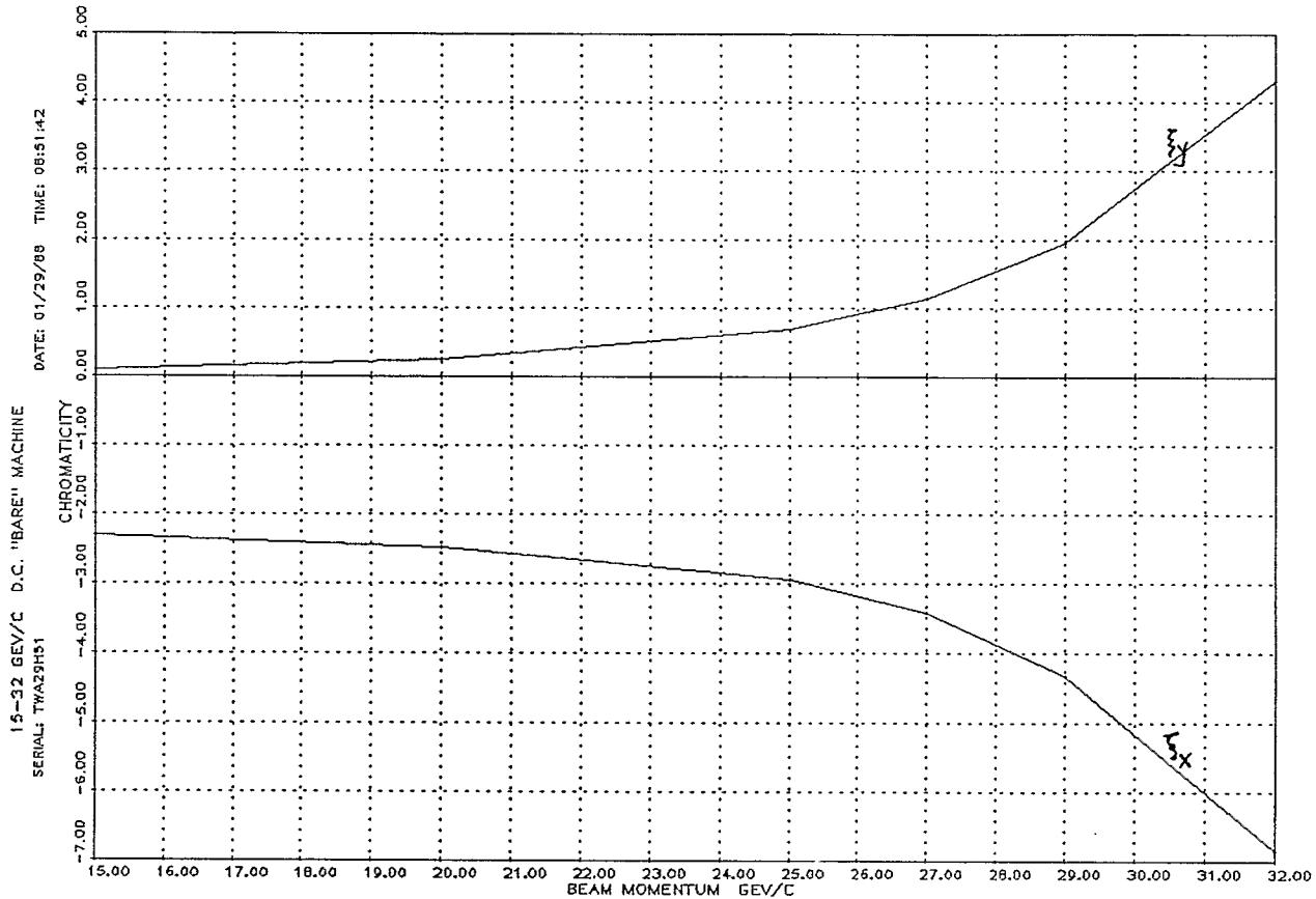
Figure 26. Energy Dependence of the Horizontal and Vertical Chromaticity for the D. C. "Bare" Machine (main magnets only) at high fields: 15-32 GeV/c.
