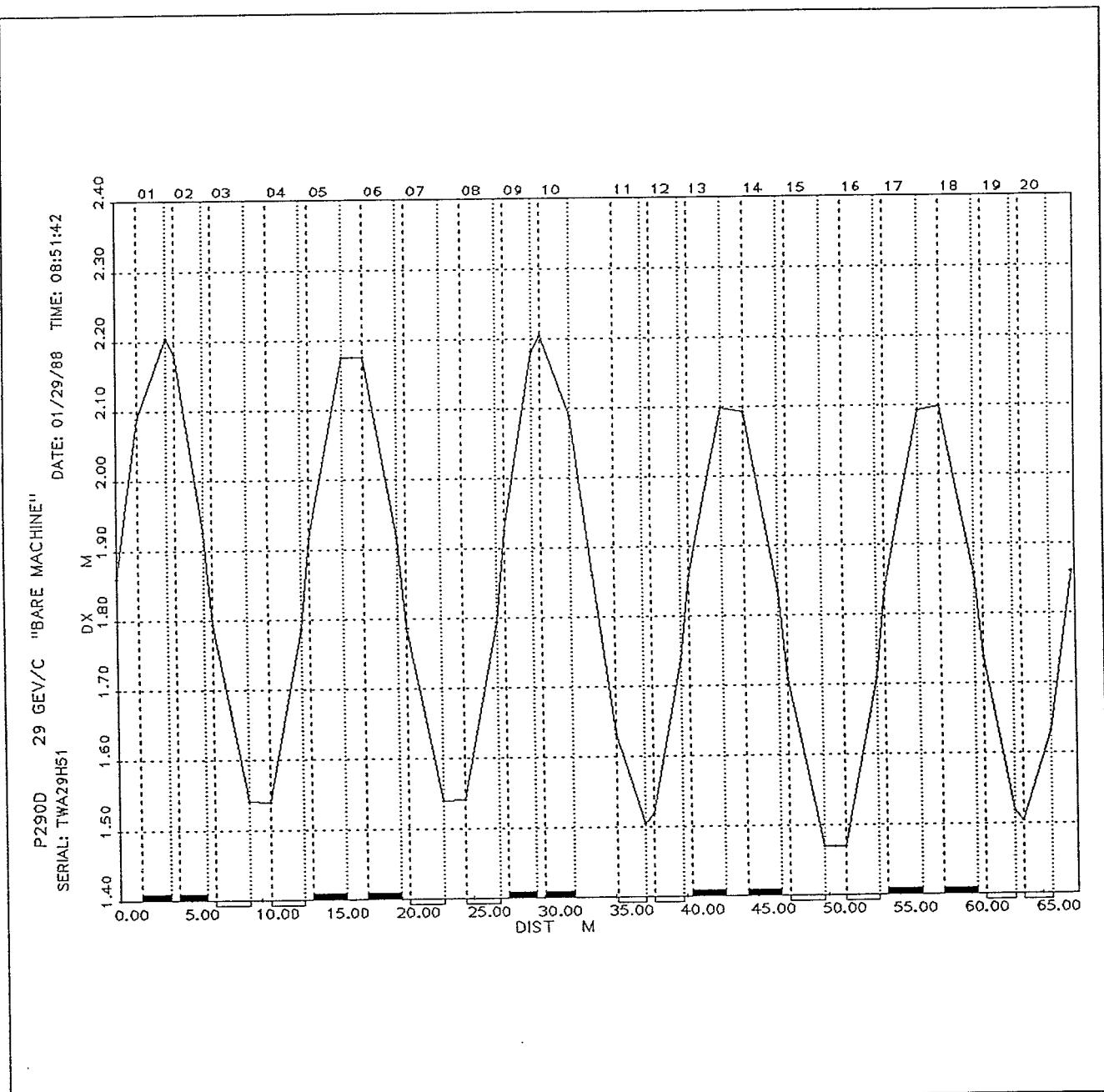
Figure 18. Dispersion Function  $dx$  (in meters) for the D. C. "Bare" Machine (main magnets only) at 29 GeV/c, given for one superperiod.
