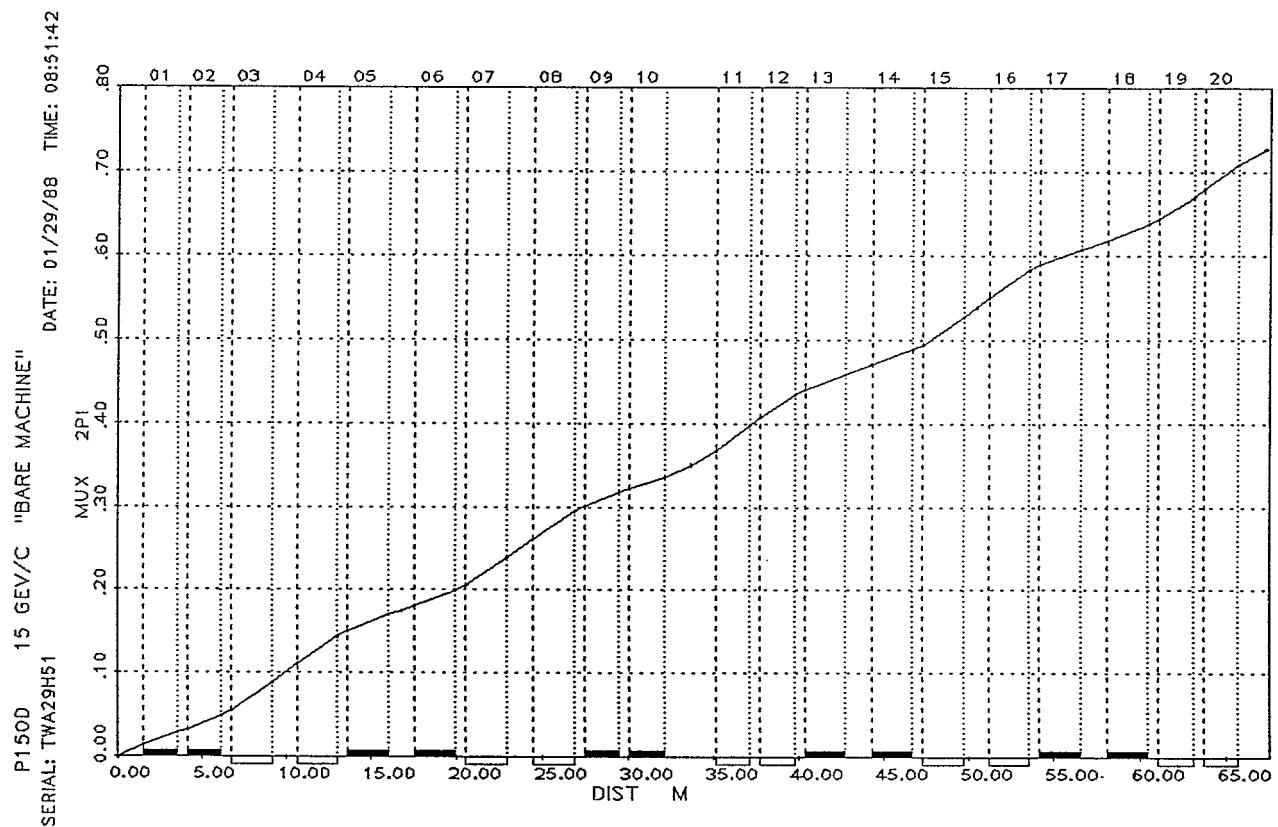
Figure 11. Phase Function  $\mu_x$  (in units of  $2\pi$  radians) for the D. C. "Bare" Machine (main magnets only) at 15 GeV/c, given for one superperiod.
