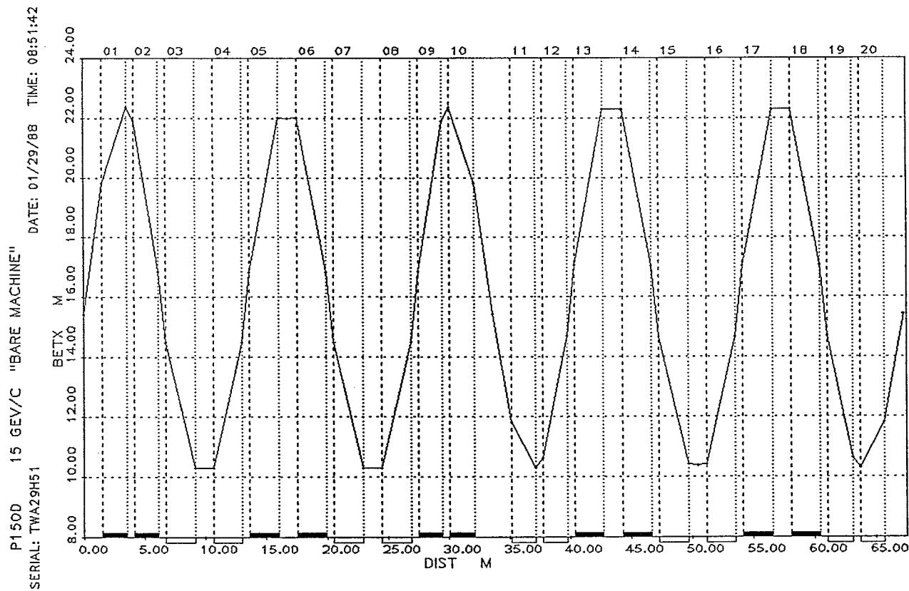
Figure 9. Courant-Snyder Parameter Beta-x (in meters) for the D. C. "Bare" Machine (main magnets only) at 15 GeV/c, given for one superperiod.
