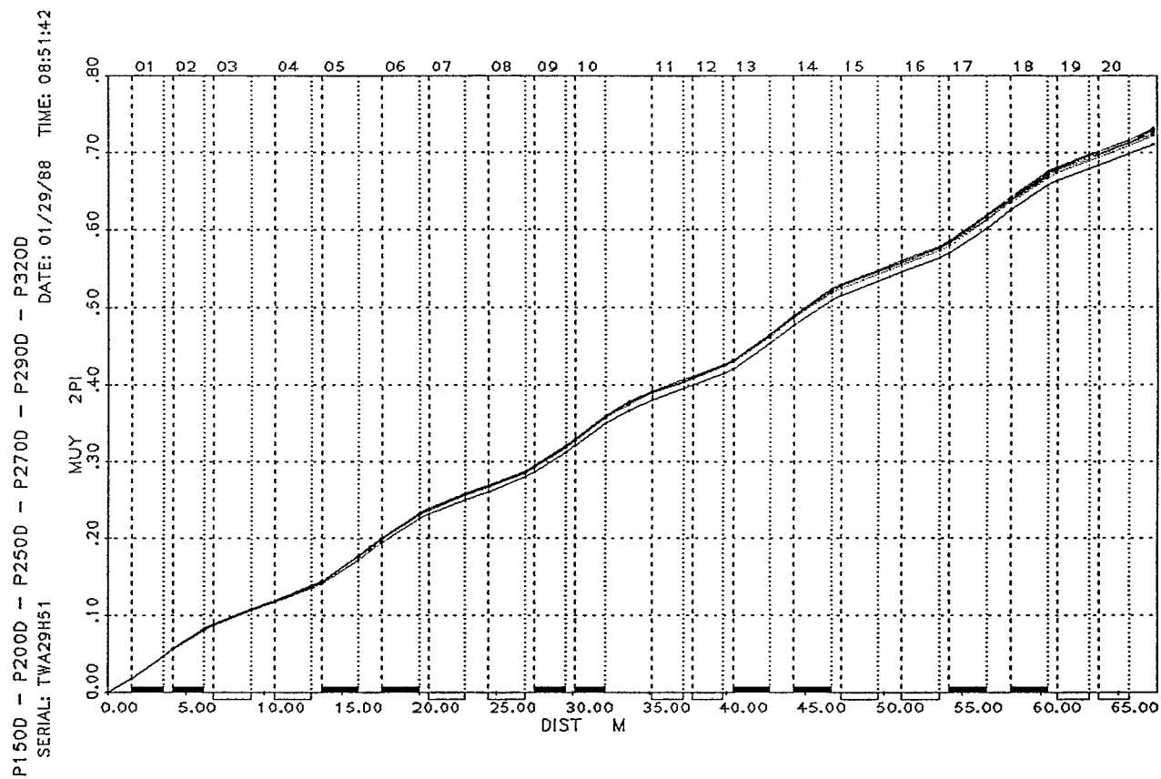
Figure 6. Phase Function  $\mu_y$  (in units of  $2\pi$  radians) for the D.C. "Bare" Machine (main magnets only) at high fields: 15-32 GeV/c, given for one superperiod.
