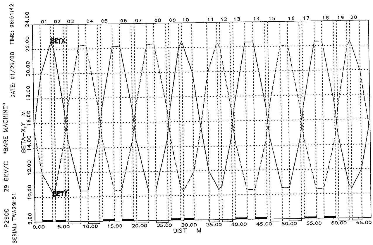
Figure 30. Courant-Snyder Parameters Beta-x and Beta-y (in meters) for the D.C. "Bare" Machine (main magnets only) at 29 GeV/c, shown on the same plot.
