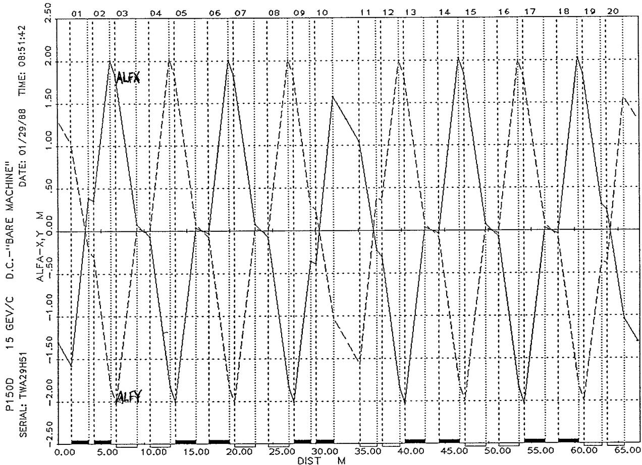
Figure 28. Courant-Snyder Parameters Alpha-x and Alpha-y (dimensionless) for the D.C. "Bare" Machine (main magnets only) at 15 GeV/c, shown on the same plot. Note that Alpha always has a negative slope in a straight section.
