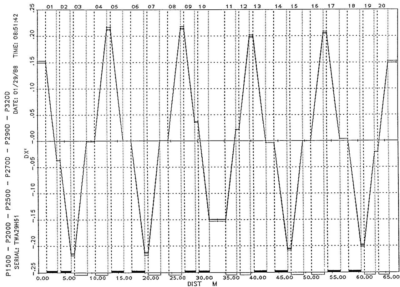
Figure 8. Derivative of Dispersion  $dx'$  (dimensionless) for the D.C. "Bare" Machine (main magnets only) at high fields: 15-32 GeV/c, given for one superperiod.
