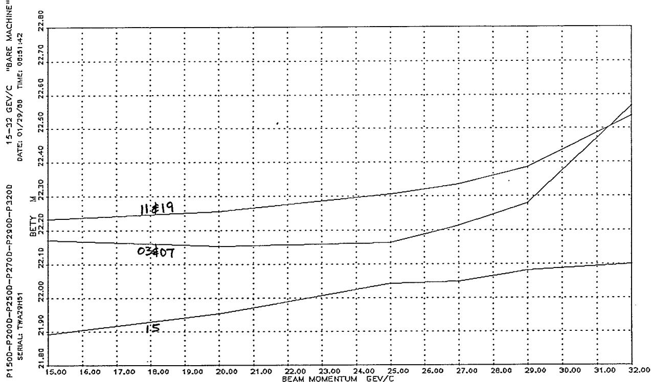
Figure 21. Energy Dependence of the Maxima in Beta-y (in meters) for the D. C. "Bare" Machine (main magnets only) at high fields: 15-32 GeV/c. (Corresponds to Figure 2.) The several maxima are labelled by the machine section in which they occur.
