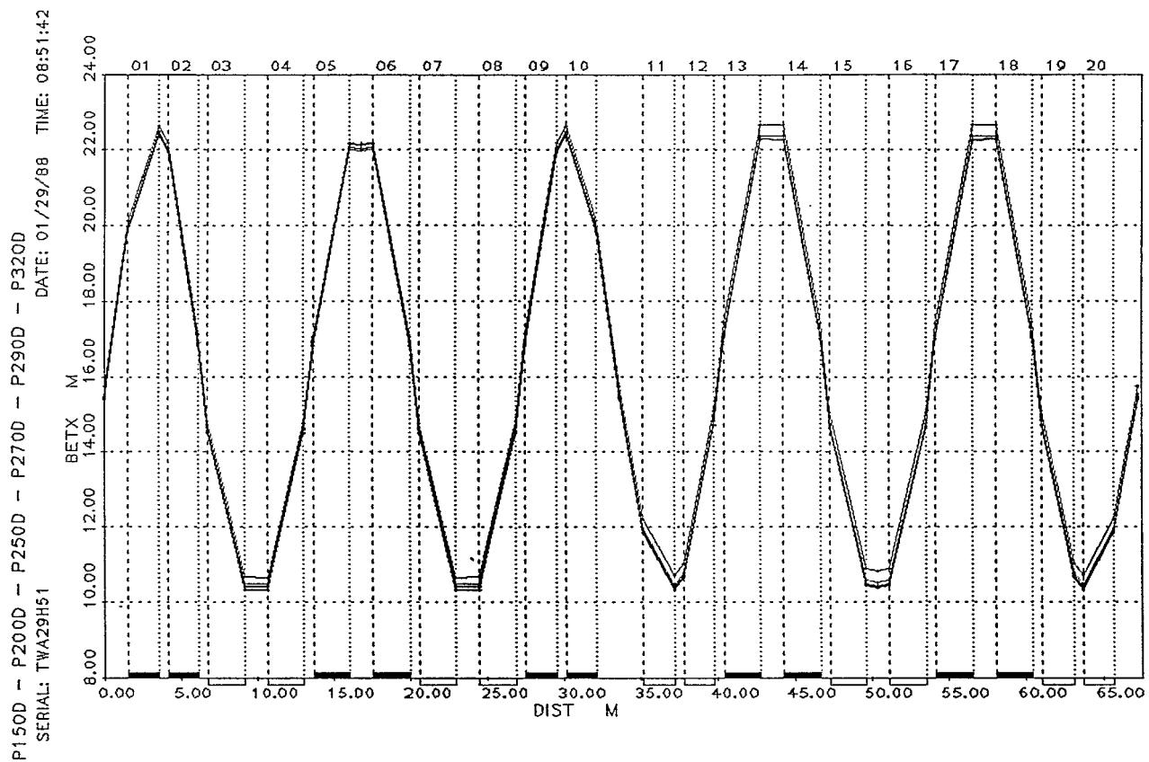
Figure 1. Courant-Snyder Parameter Beta-x (in meters) for the D.C. "Bare" Machine (main magnets only) at high fields: 15-32 GeV/c, given for one superperiod.
