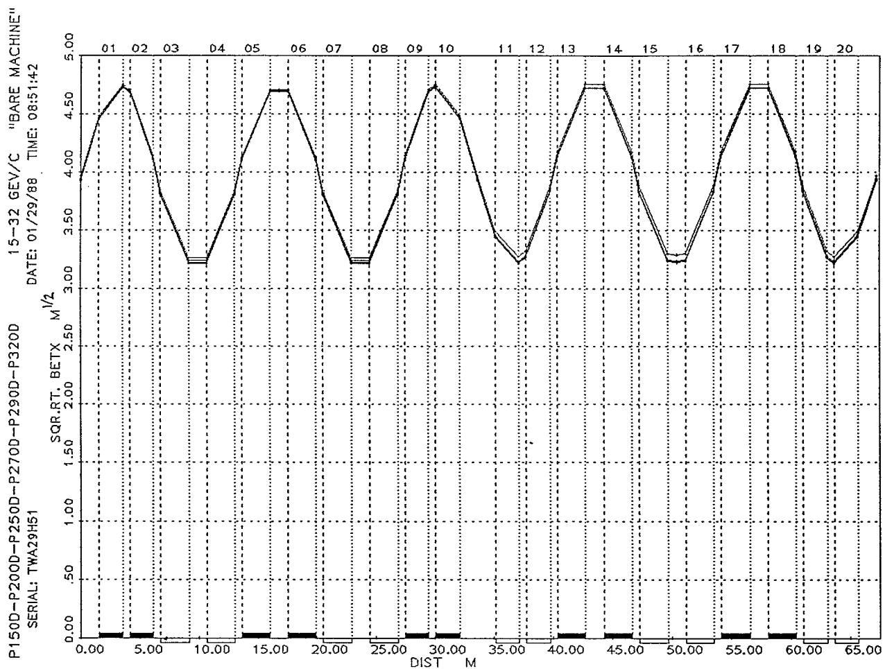
Figure 33. Courant-Snyder Parameter Beta-x shown on a square root scale for the D.C. "Bare" Machine (main magnets only) at high fields: 15-32 GeV/c, given for one superperiod. (Corresponds to Figure 1 which has a linear scale.)
