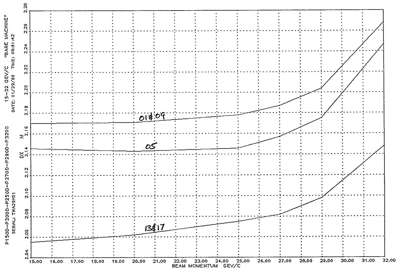
Figure 23. Energy Dependence of the Maxima in Dispersion (in meters) for the D. C. "Bare" Machine (main magnets only) at high fields: 15-32 GeV/c. (Corresponds to Figure 7.) The several maxima are labelled by the machine section in which they occur.
