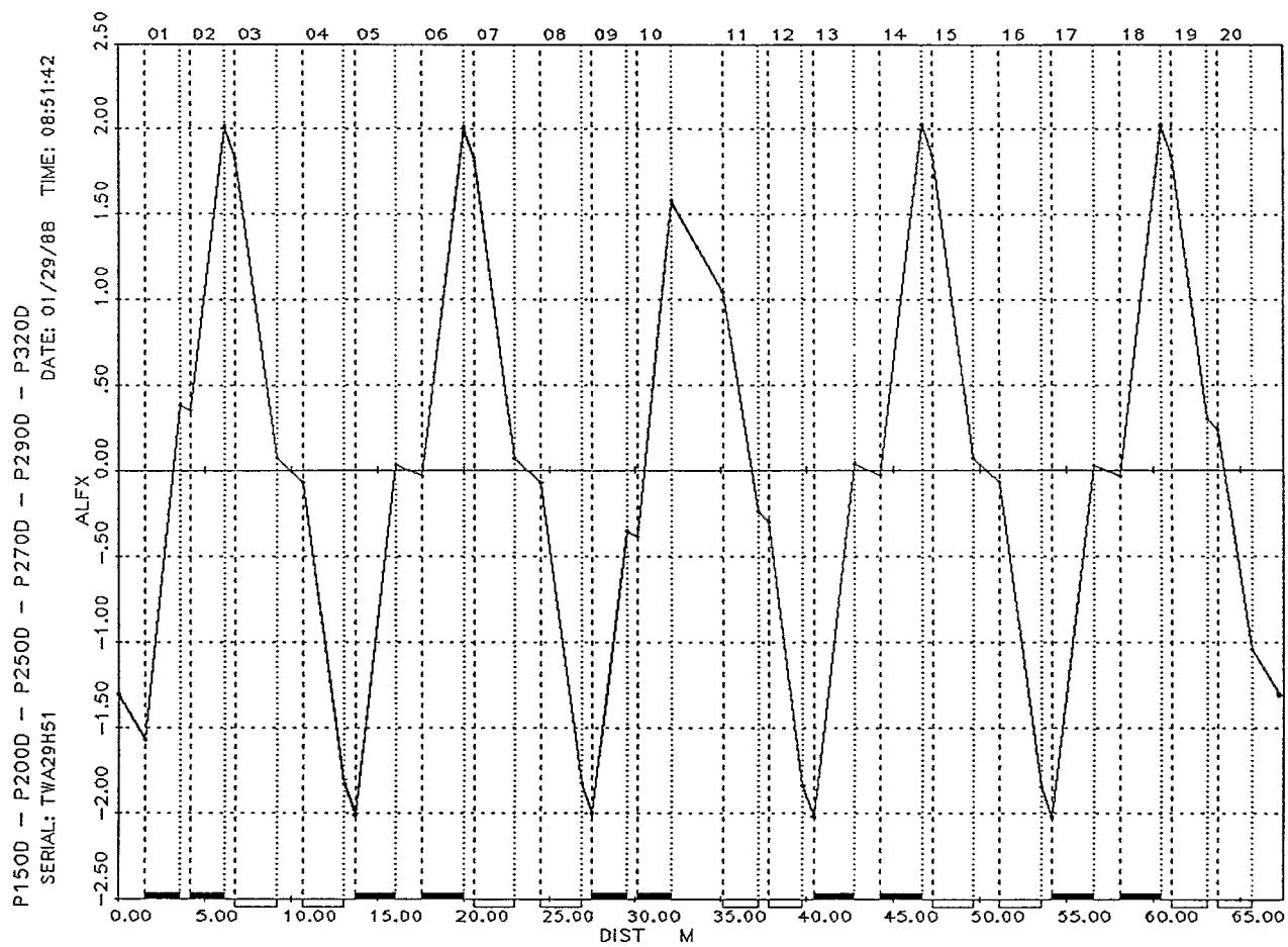
Figure 3. Courant-Snyder Parameter Alpha-x (dimensionless) for the D. C. "Bare" Machine (main magnets only) at high fields: 15-32 GeV/c, given for one superperiod.
