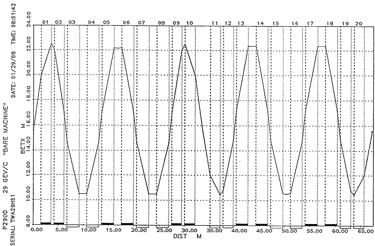
Figure 14. Courant-Snyder Parameter Beta-x (in meters) for the D. C. "Bare" Machine (main magnets only) at 29 Gev/c, given for one superperiod.
