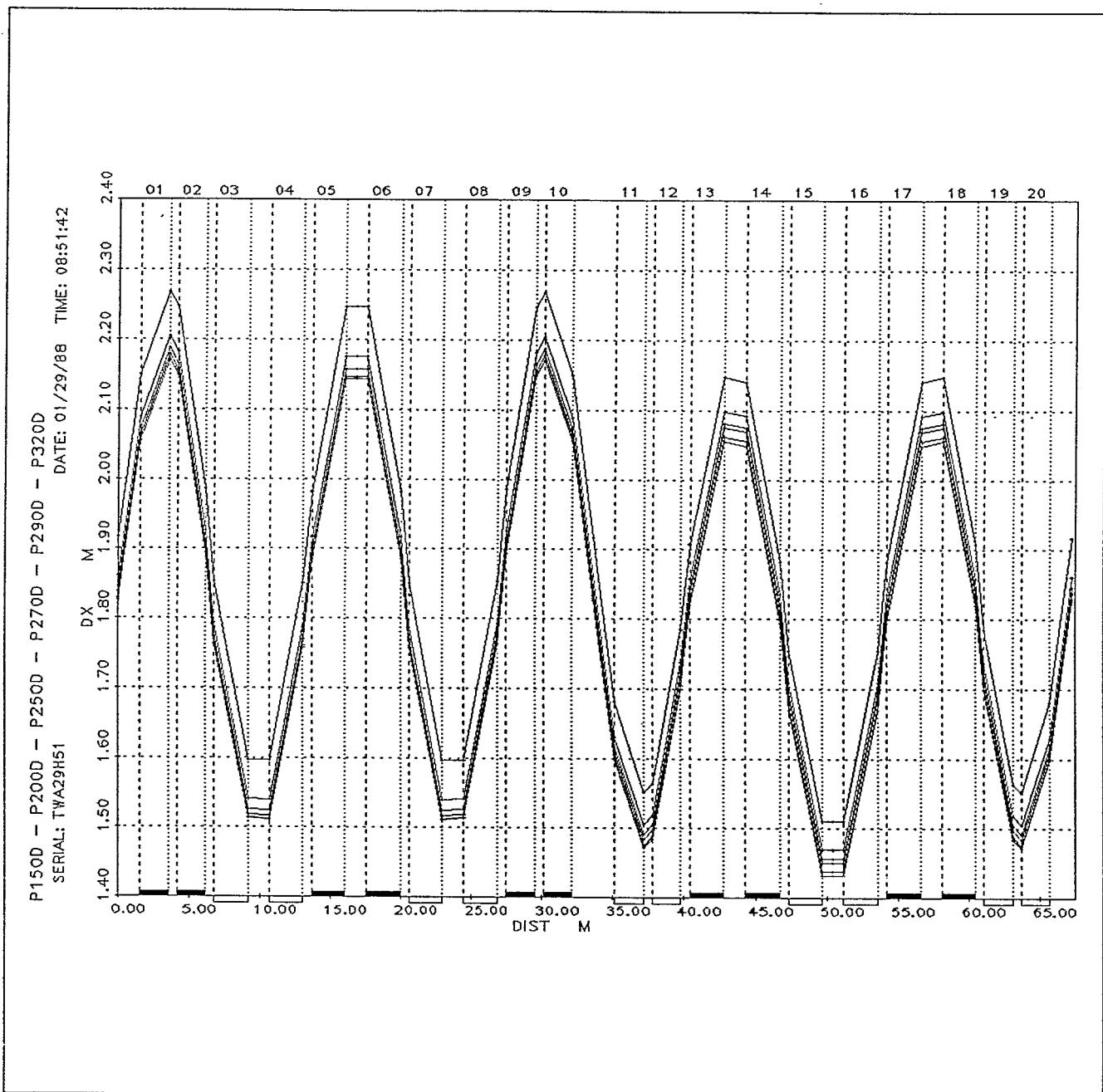
Figure 7. Dispersion Function  $dx$  (in meters) for the D.C.
