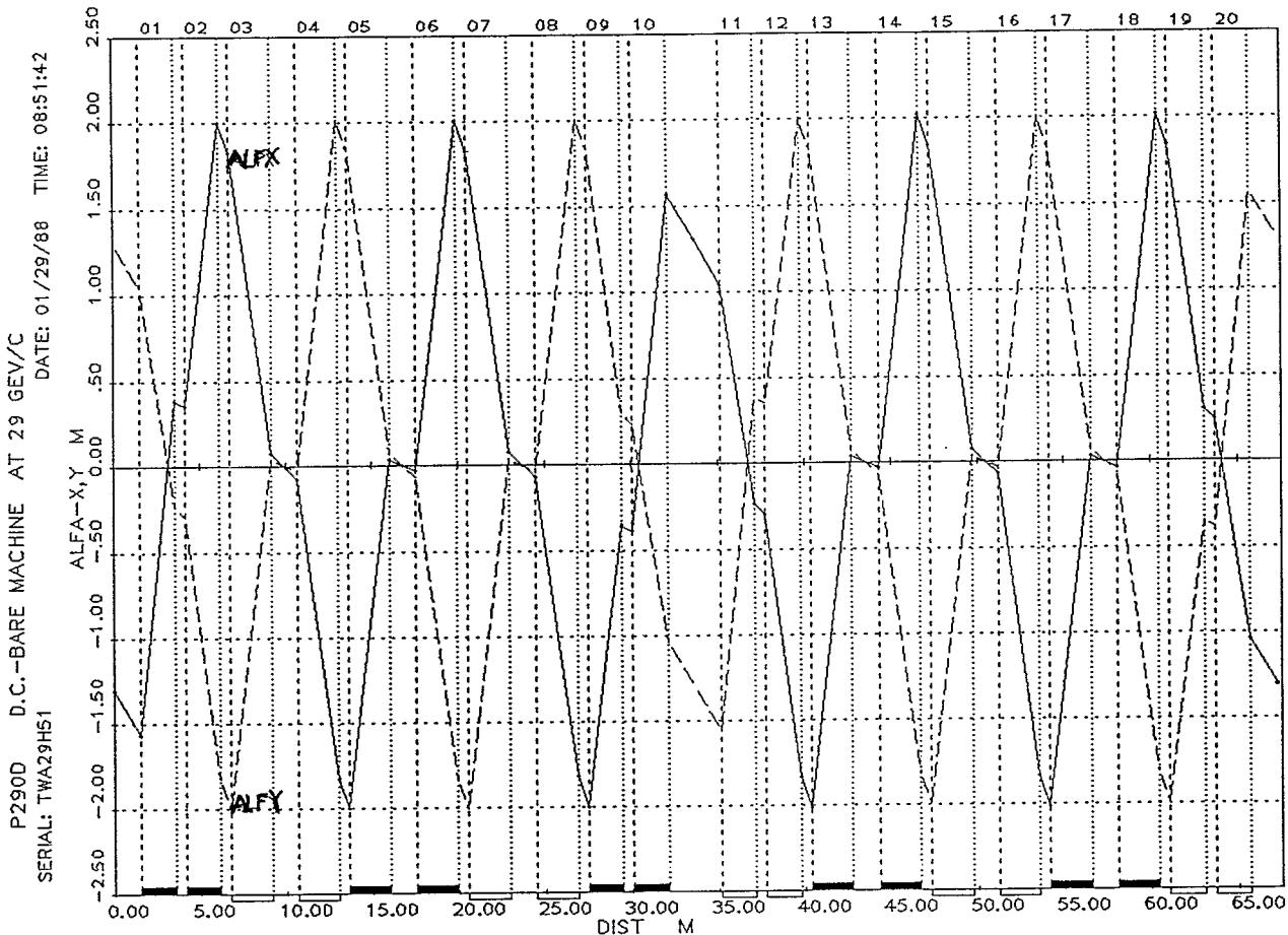
Figure 31. Courant-Snyder Parameters Alpha-x and Alpha-y (dimensionless) for the D.C. "Bare" Machine (main magnets only) at 29 GeV/c, shown on the same plot. Note that Alpha always has a negative slope in a straight section.
