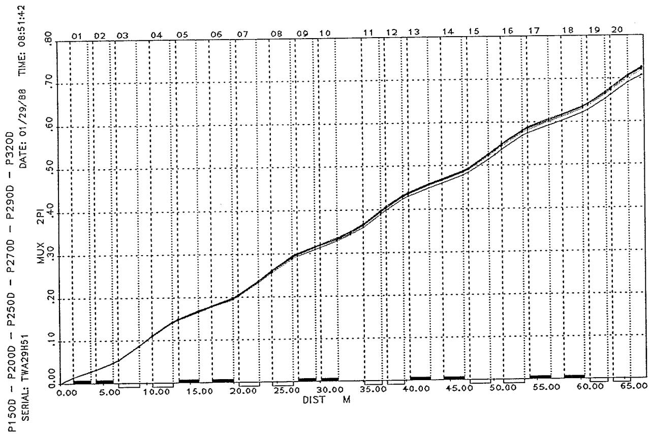
Figure 5. Phase Function Mu-x (in units of  $2\pi$  radians) for the D.C. "Bare" Machine (main magnets only) at high fields: 15-32 GeV/c, given for one superperiod.
