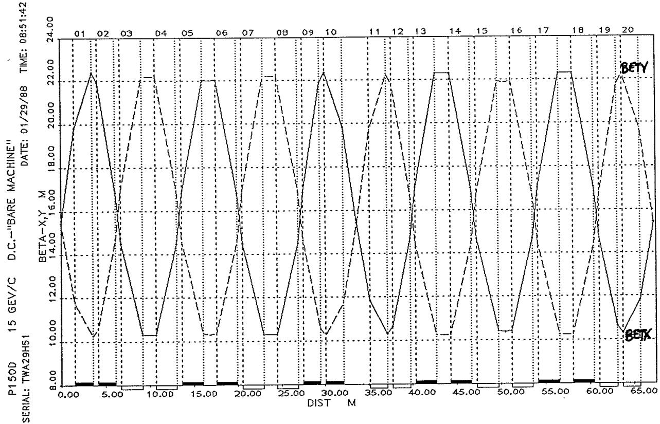
Figure 27. Courant-Snyder Parameters Beta-x and Beta-y (in meters) for the D.C. "Bare" Machine (main magnets only) at 15 GeV/c, shown on the same plot.
