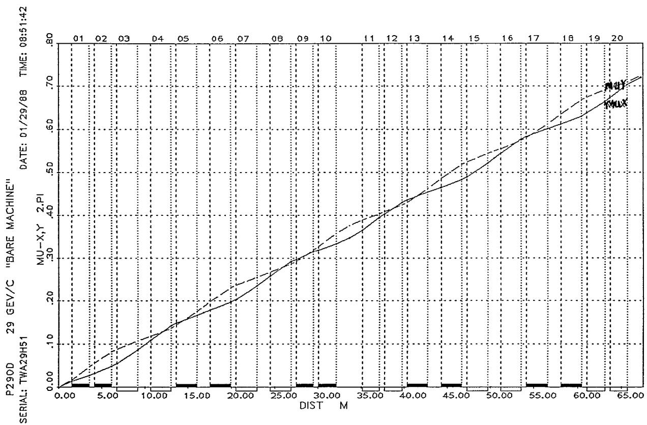
Figure 32. Phase Functions  $\text{Mu-}x$  and  $\text{Mu-}y$  (in units of  $2\pi$  radians) for the D.C."Bare" Machine (main magnets only) at 29 GeV/c, shown on the same plot. Note that only phase advance is meaningful. A different choice of zero-point would result in an upward or downward displacement of  $\text{Mu-}x$  relative to  $\text{Mu-}y$ .
