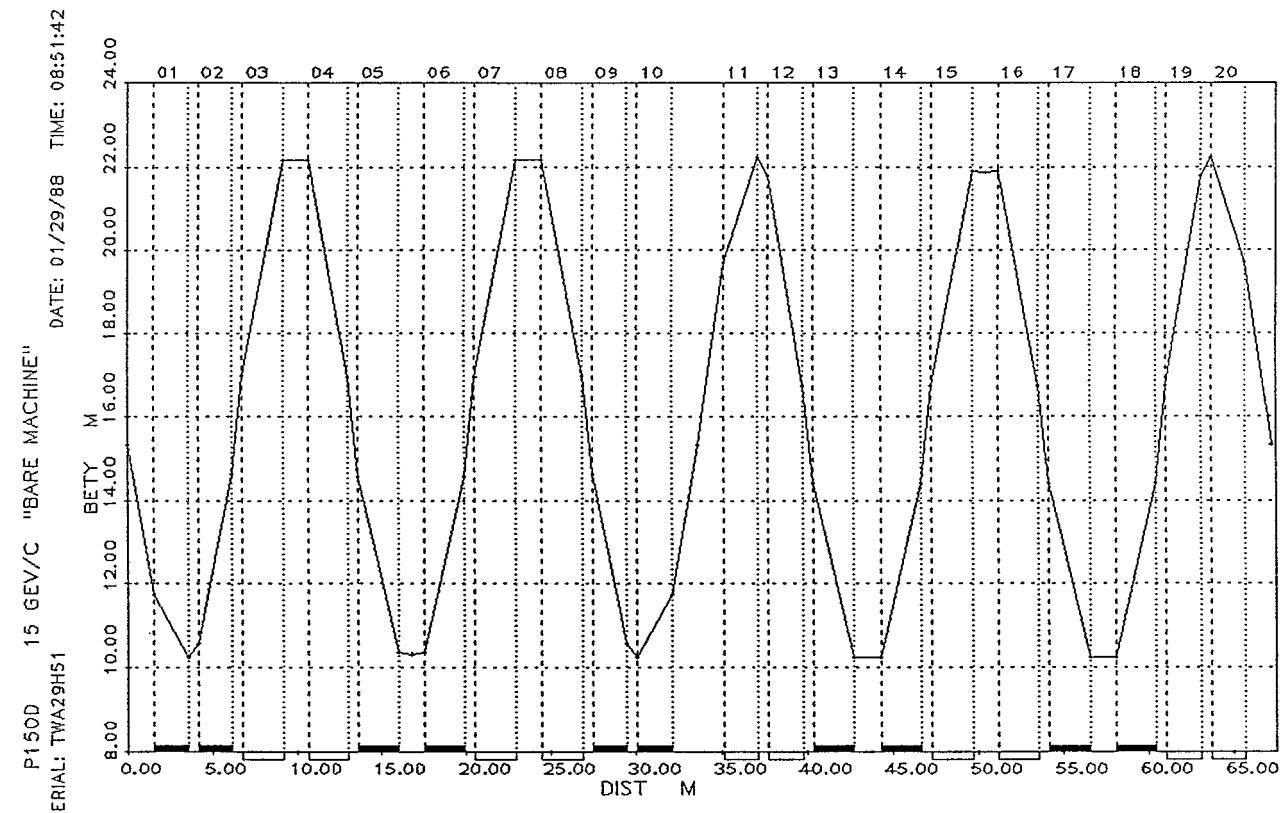
Figure 10. Courant-Snyder Parameter Beta-y (in meters) for the D. C. "Bare" Machine (main magnets only) at 15 GeV/c, given for one superperiod.
