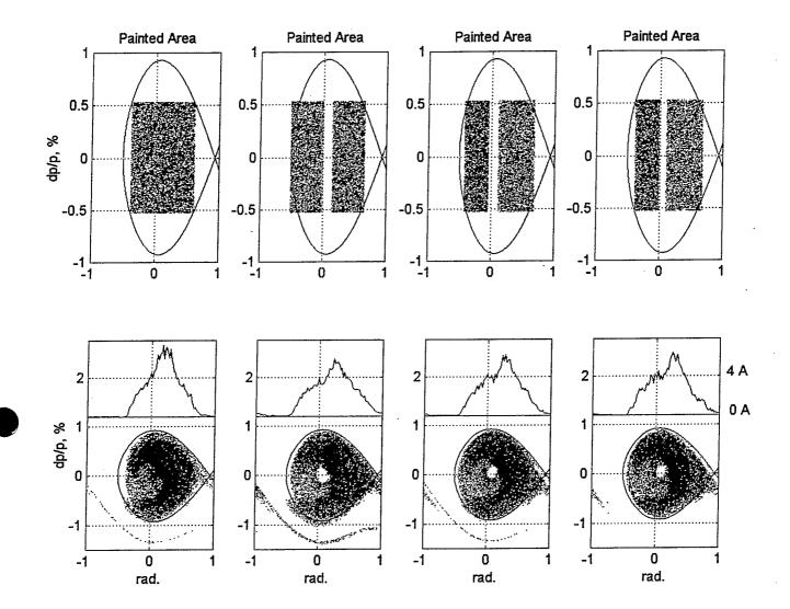
Fig.9. Injection with manipulation of fast chopper, cutting the middle of the beam.
