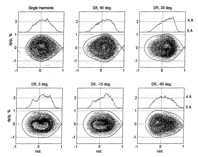
V=90 KV, Chopper 180 deg. shifted 15 deg. 15 TP, 360 turns, Bdot 3.4-3.6 T/s
