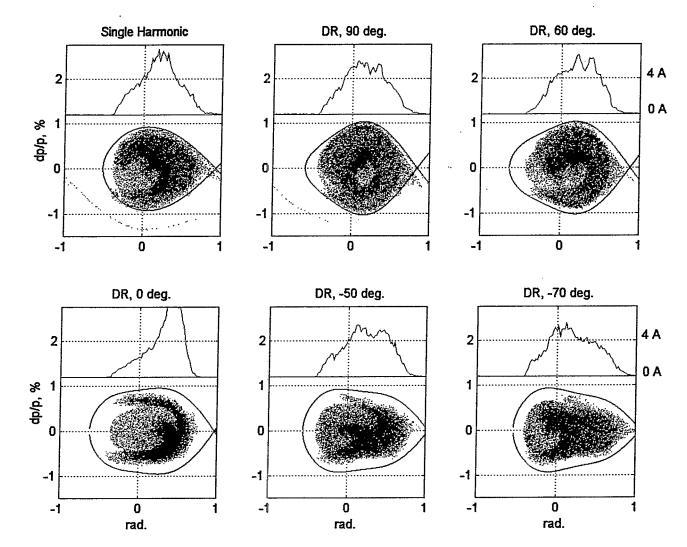
V=45 KV, Chopper 180 deg. shifted 22 deg. 15 TP, 360 turns, Bdot 3.4-3.6 T/s
