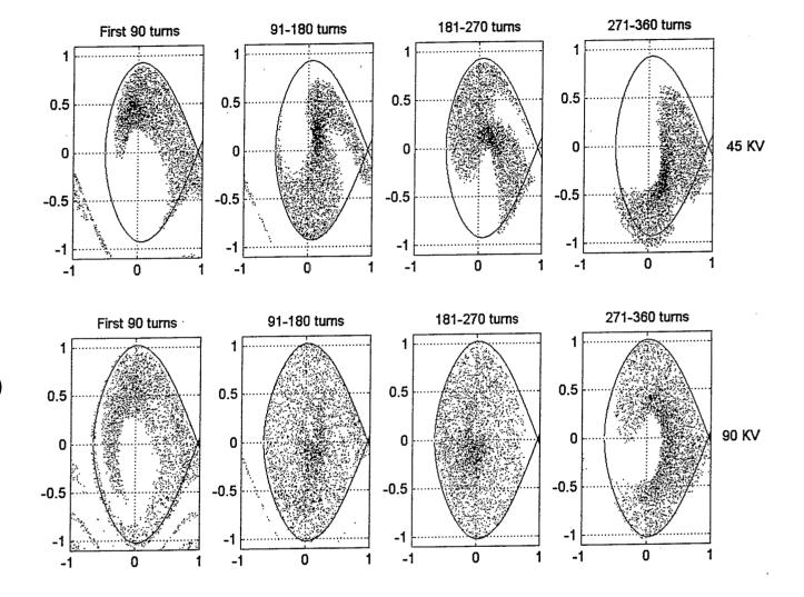
Fig.2. Particle distribution at the end of stacking, for each 90 turns, for  $V_{RF} = 45 \text{ KV}$ , h = 1 and  $V_{RF} = 90 \text{ KV}$ , h = 2
