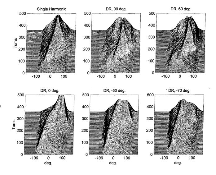
Fig.6. Mountain range of double RF with difference phase,  $V_{RF} = 45 \ KV, \ h = 1.$
