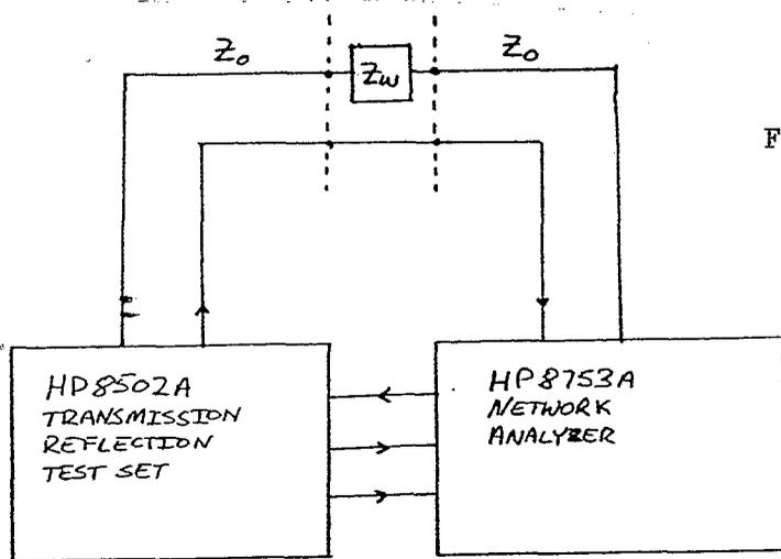
Fig. 2. Test setup used to measure S21.
