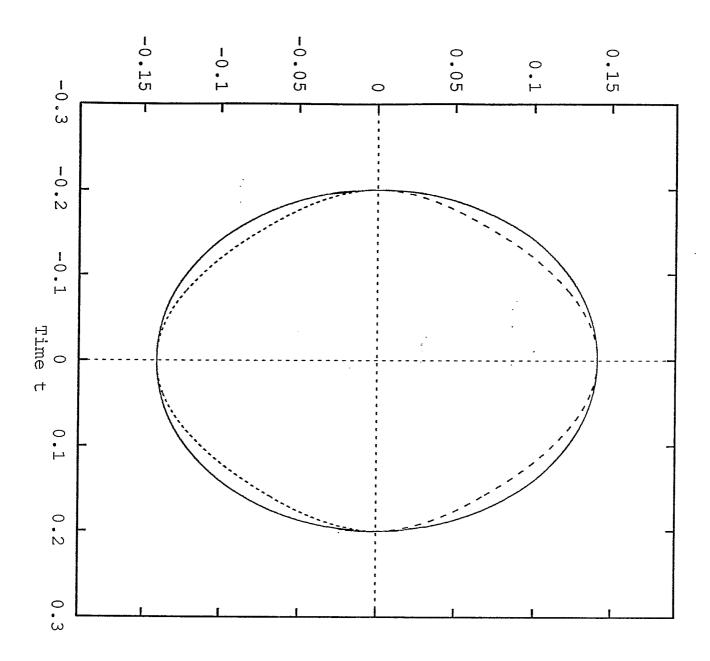
Figure 2: Bunch shape in the first synchrotron (in solid line). Phase trajectory of point  $(t_{i2}, 0)$  in the second synchrotron to find the nominal matching voltage (in dash line).
