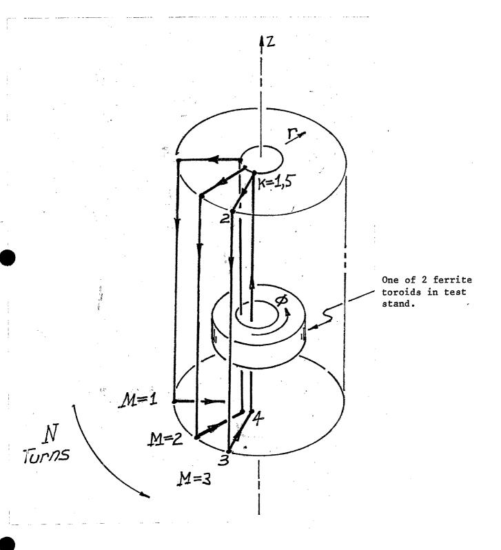
Figure 3. N-turn tuning coil geometry.
