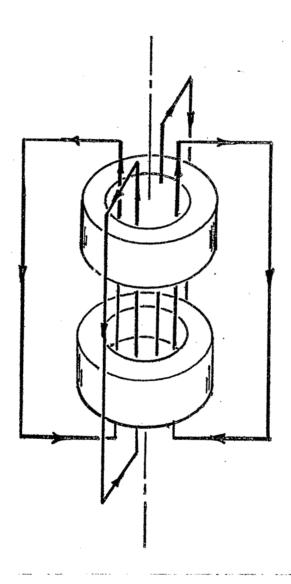
Figure 1. Four-turn tuning coil geometry.
