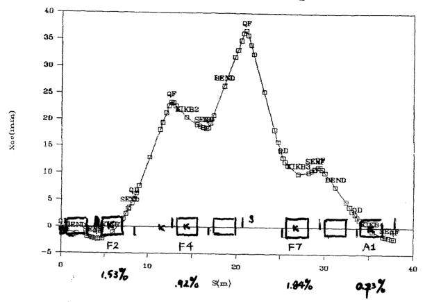
Fig. 1 An example of orbit bump backley winding.
