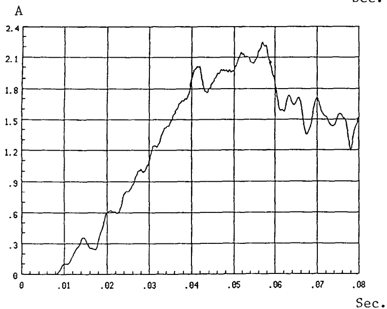
Magnet Current Error Due to 8ms 1% Step Power Line Disturbance
