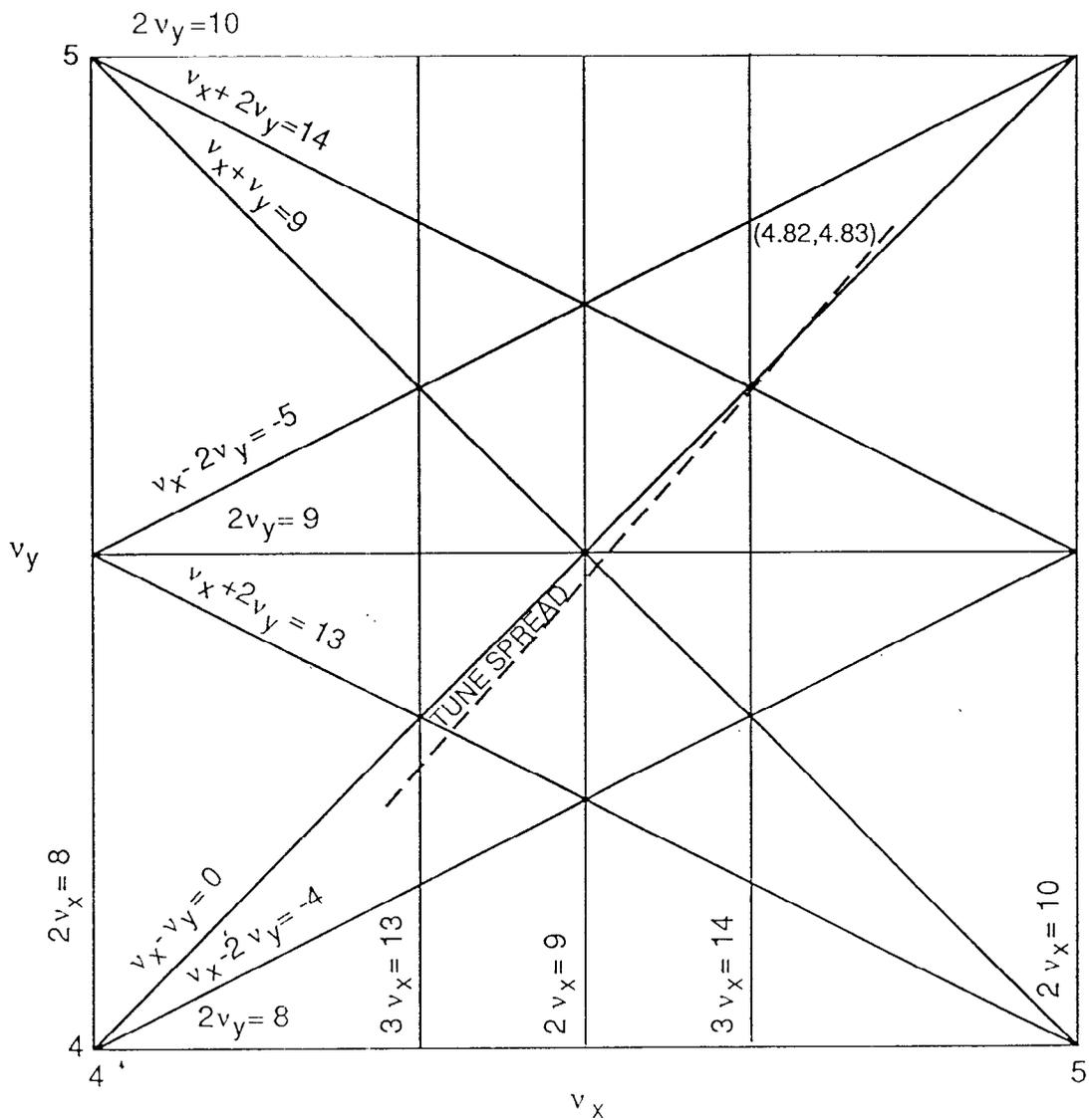
Fig. 1. The Tune diagram with the expected tune spread from space charge<sup>1</sup>
