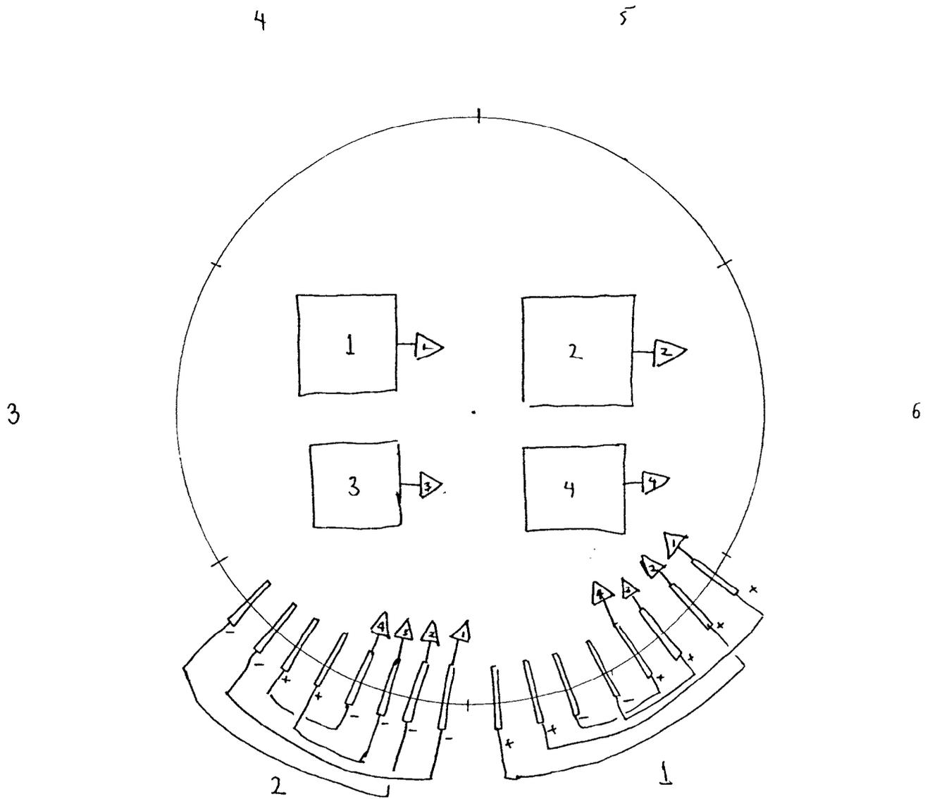
Fig 2. Power supply configuration for the Quadrupole correctors. Note, superperiod pairs (3,4) and (5,6) are identical to (1,2). The + and - signs indicate the direction of current through the coils.
