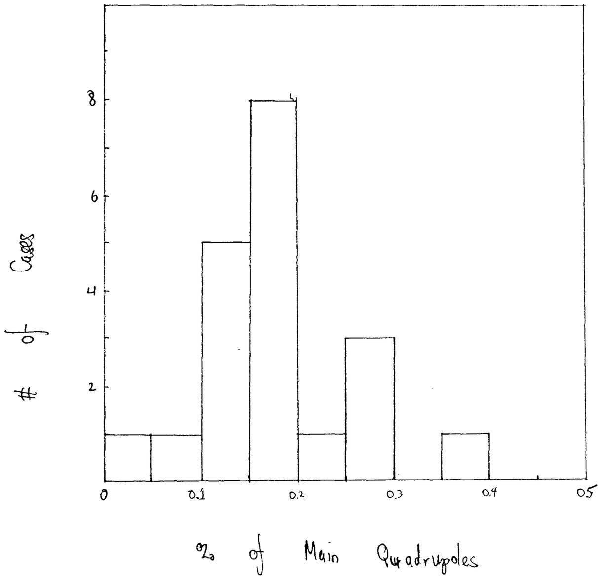
Fig. 5. The distribution of the maximum skew quadrupole corrector strength over the 20 cases tried.
