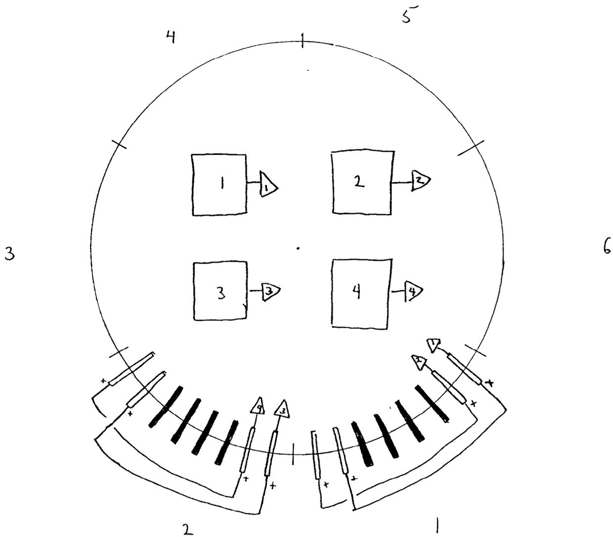
Fig. 4 The power supply configuration for the skew quadrupole correctors. Note, superperiods <sup>pairs</sup> (3, 4) and (5, 6) are connected identically as (1, 2). The + and - signs indicate the direction of current through the coils. Additionally, there are only 4 skew quadrupole correctors per superperiod.
