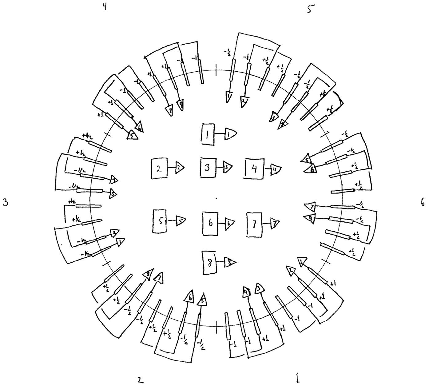
Fig. 6 The power supply configuration for the sextupole correctors. Note, some of the correctors are powered at  $\frac{1}{2}$  the strength.
