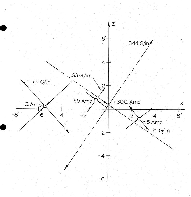
Fig. 1 Axis and field gradients of skew quadrupole at E15. Axis is defined as point of zero field. X, Z is a system of coordinates whose origin is within 100 mils of the physical center of quadrupole.
