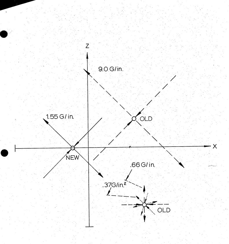
Fig. 2 Axis of old and new quadrupole magnets. The dashed and dotted vectors indicate the quadrupole and sextupole field gradients of the old magnet respectively. Two zero field points were found in this magnet.
