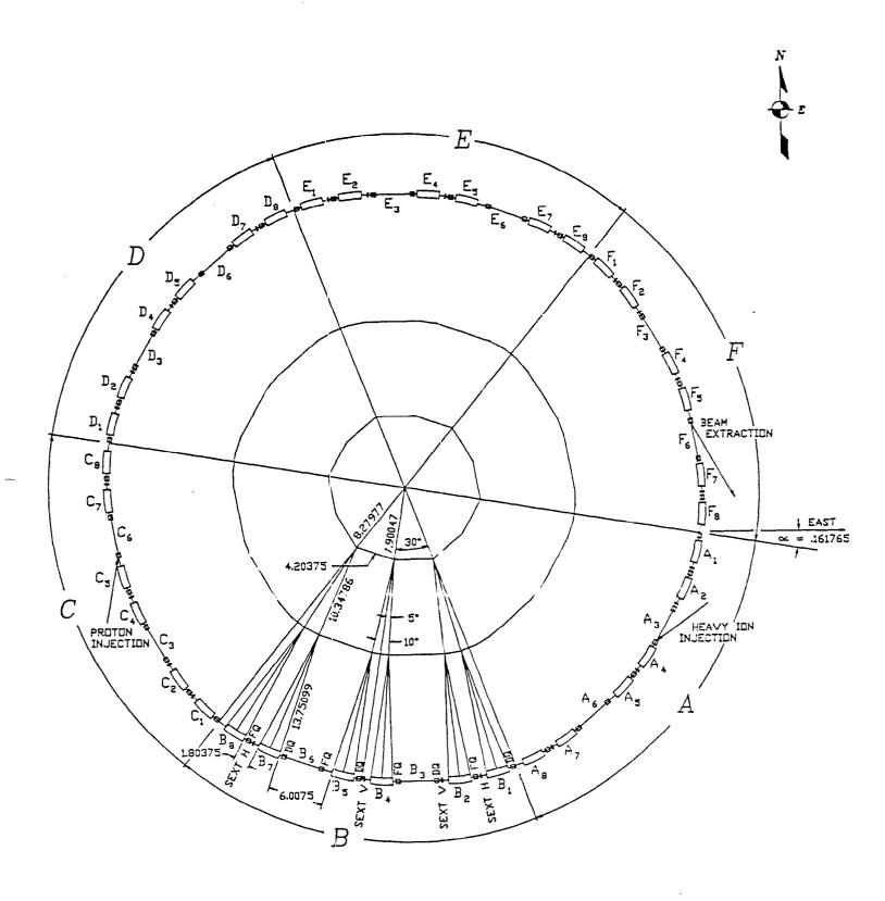
Fig. 1 The Booster Lattice
