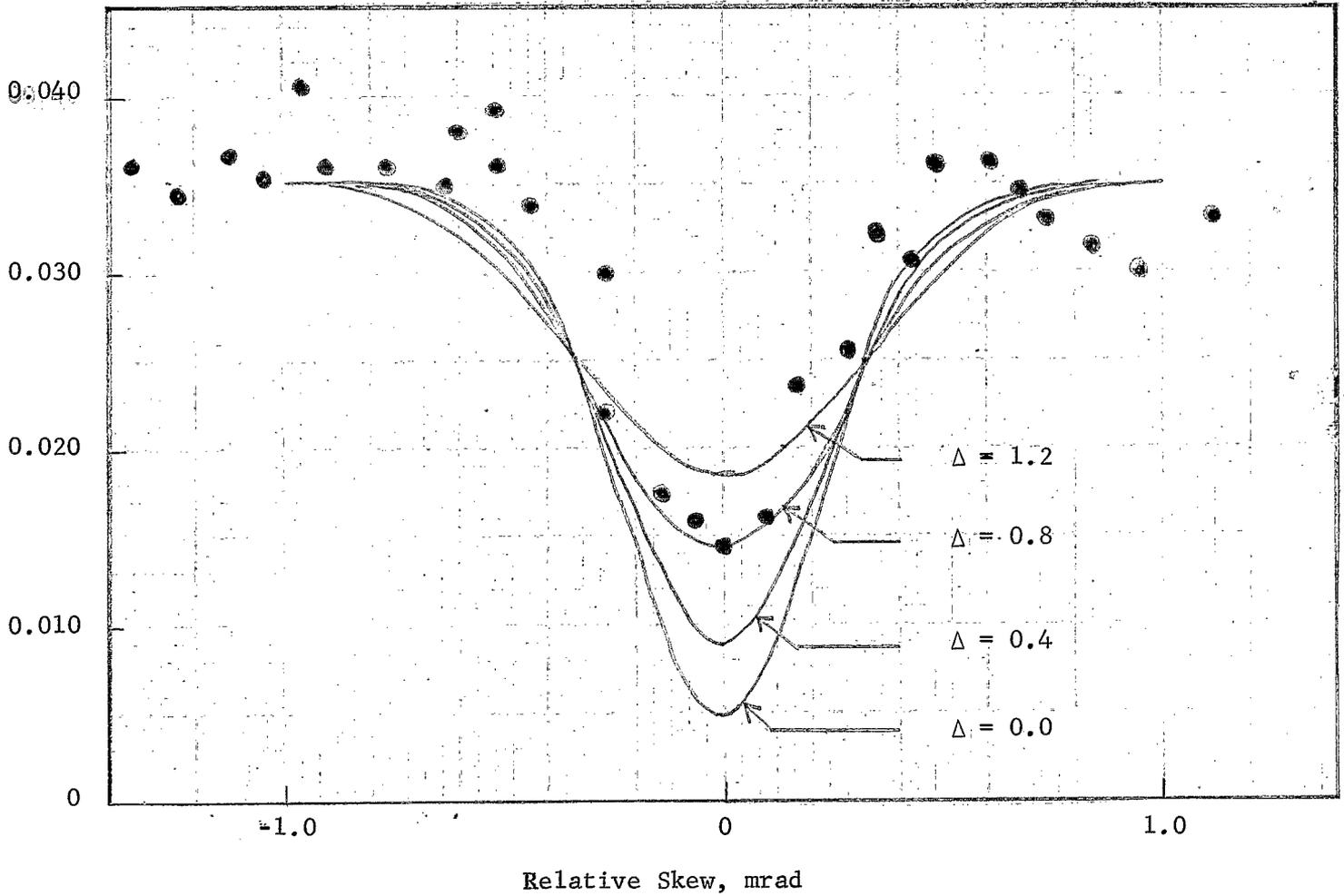
Fig. 3 Loss monitor signal vs. septum skew angle. The points are measured values (background subtracted). The curves are predictions of Monte Carlo calculations for various assumed beam divergences  $\Delta$  in milliradians.
