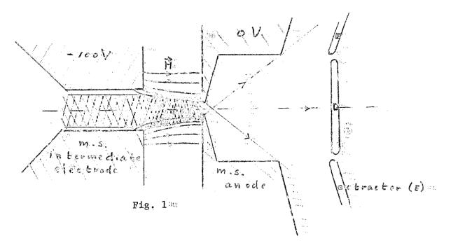
It is caused by the amplification of ionization towards the anode of increased electron energy) and contraction of the plasma by the non-uniform magnetic field. This configuration forms a high concentration of charged particles just sinside or in front of the anode aperture.
