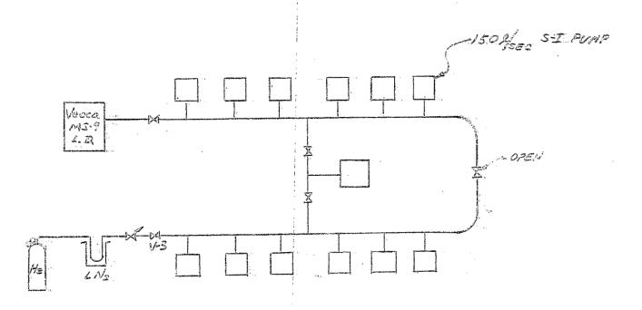
The system was pumped to a base pressure, valve V-3 was opened and the time recorded until a signal response was noted on the leak detector.
