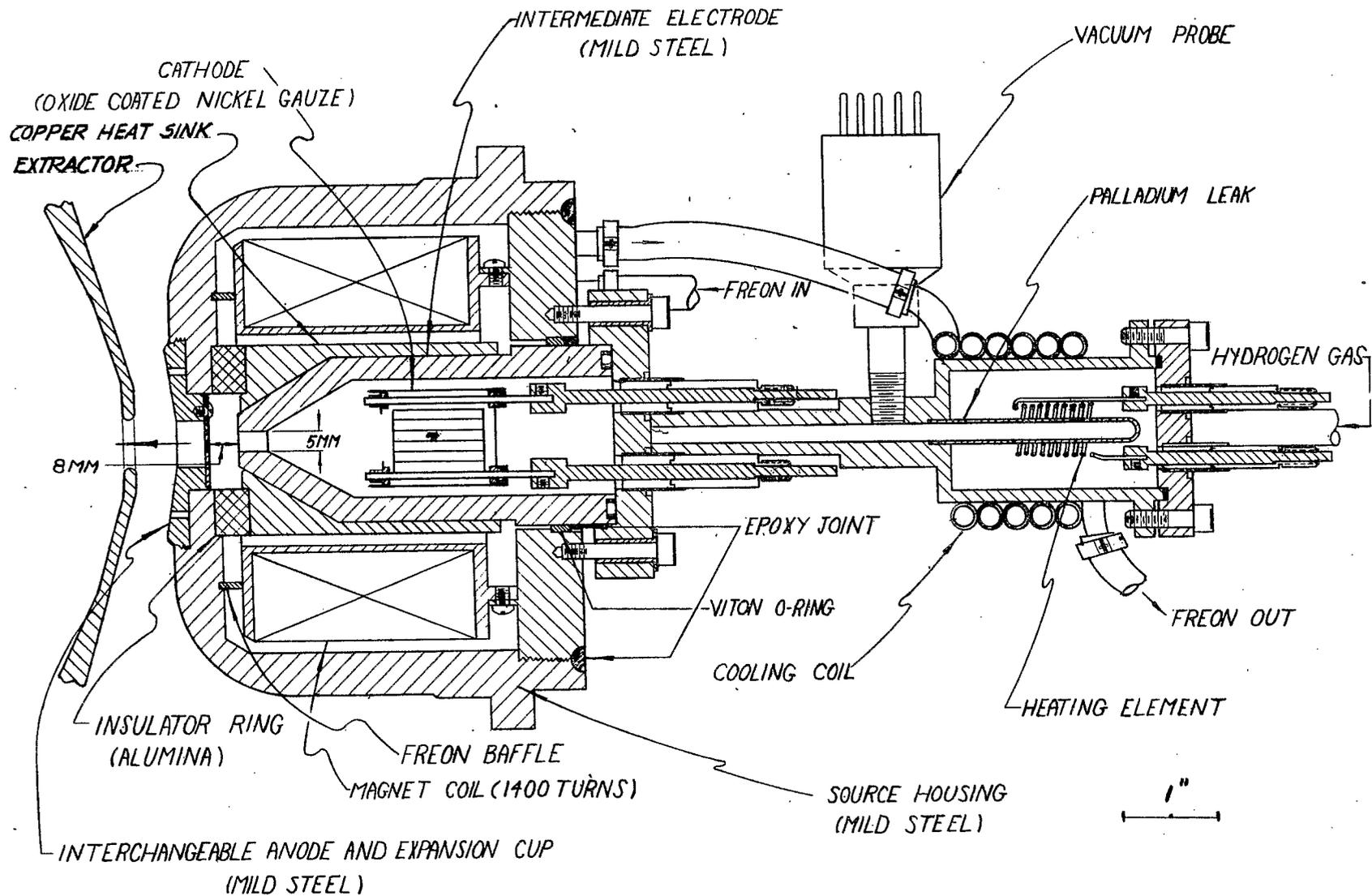
**FIG. 1** THE DUOPLASMATRON ION SOURCE AND EXTRACTOR
