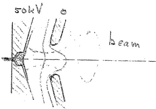
Fig. 7c Potential lines in the source test rig.
